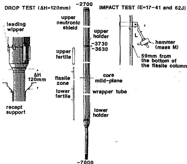
Fig. 7. Mechanical testing on irradiated PHENIX sub-assembly.
