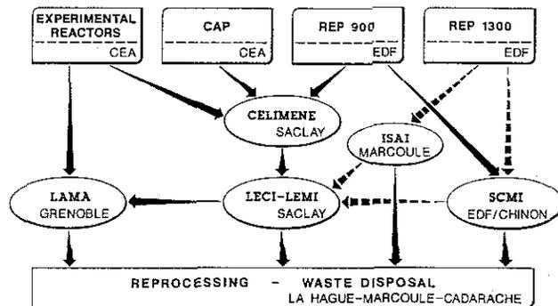
Fig.1. Examination hot cell facilities in the french P.W.R. cycle.
