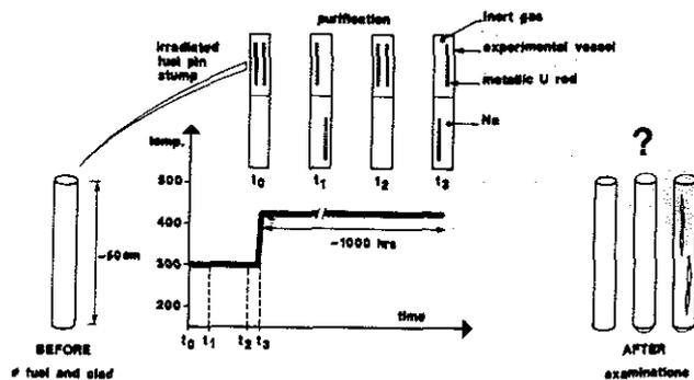
Fig. 8. Irradiated fuel/Na reaction studies "internal storage program".
