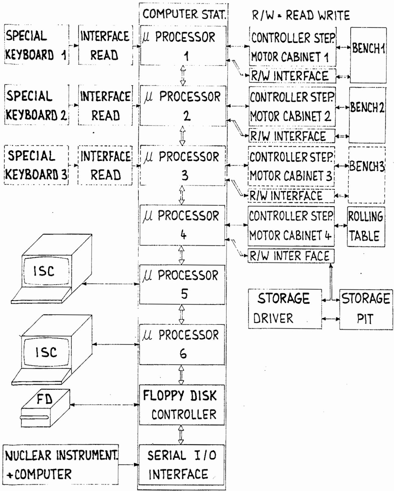
FIG.10 INSTALLATION BLOCK DIAGRAM
