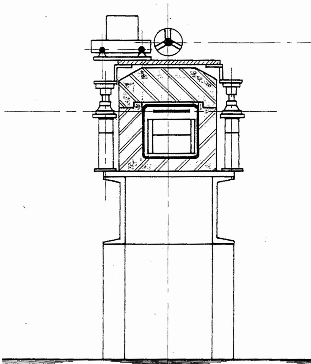
FIG.5 FILM CASSETTE TUNNEL WITH SHIELDING AND SUPPORTS
