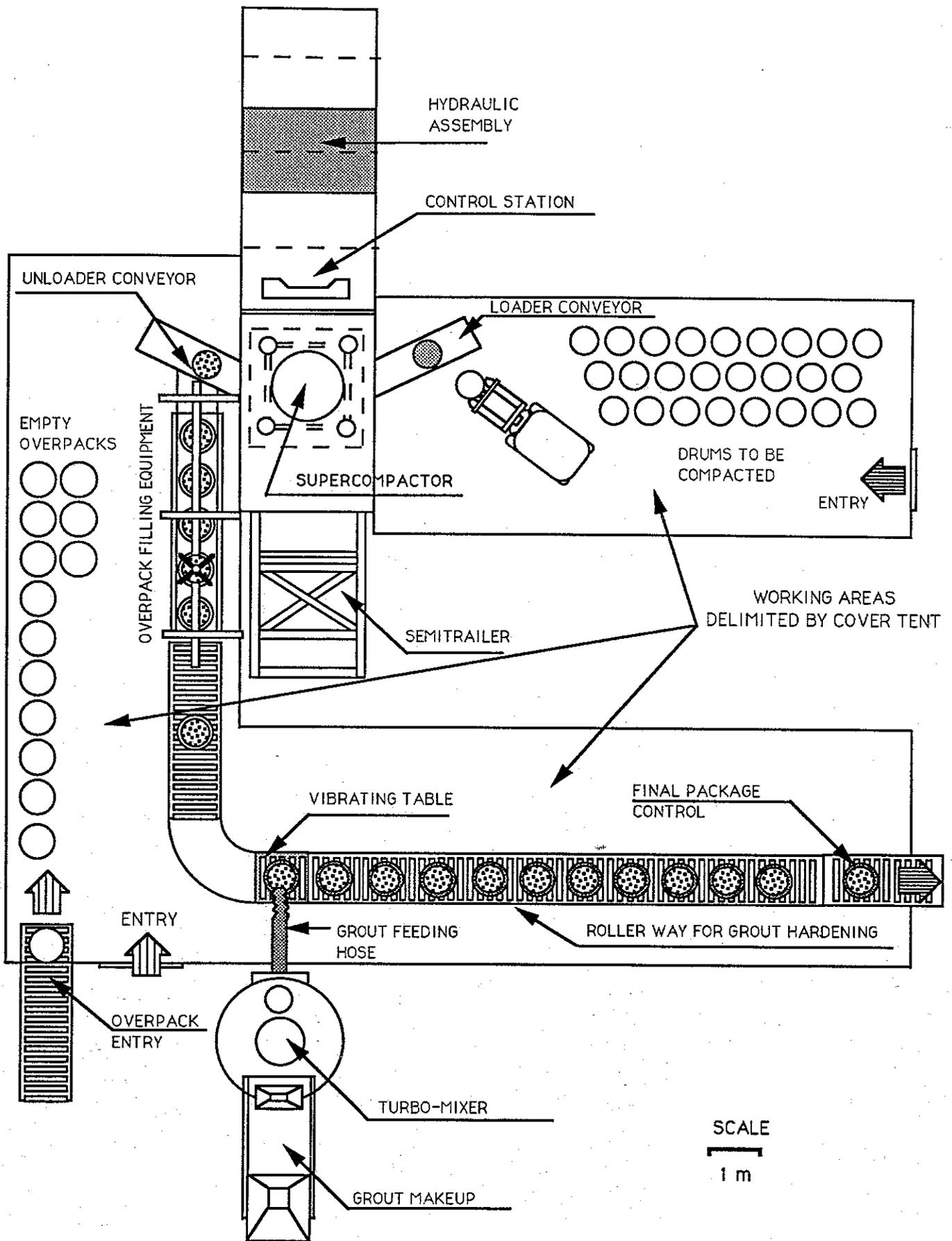
Fig. 6.1 Process lay-out of the supercompaction and conditioning facility at the ENEA Trisaia Center
