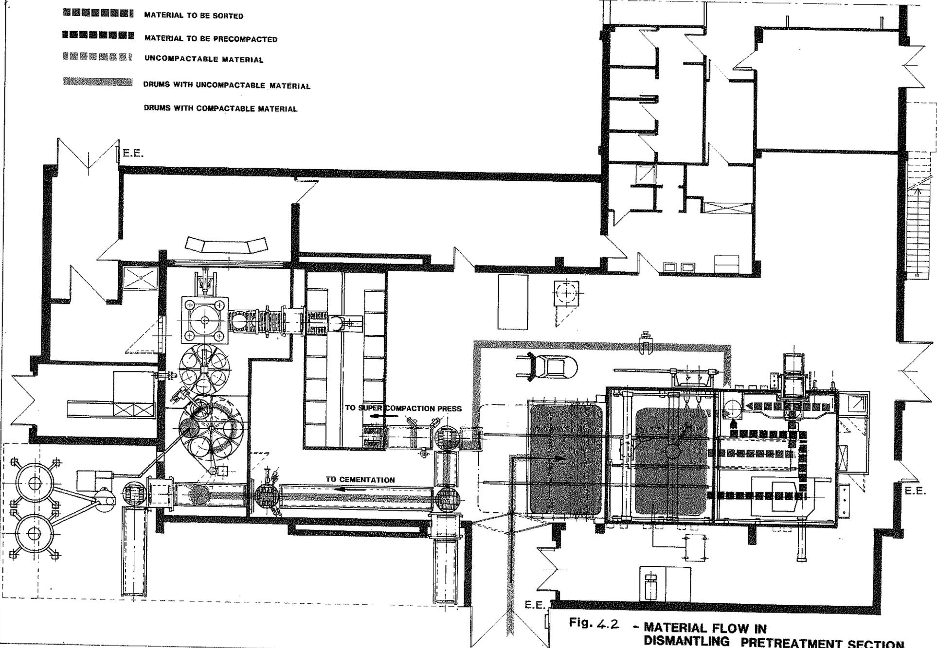
Fig. 4.2 - MATERIAL FLOW IN DISMANTLING PRETREATMENT SECTION
