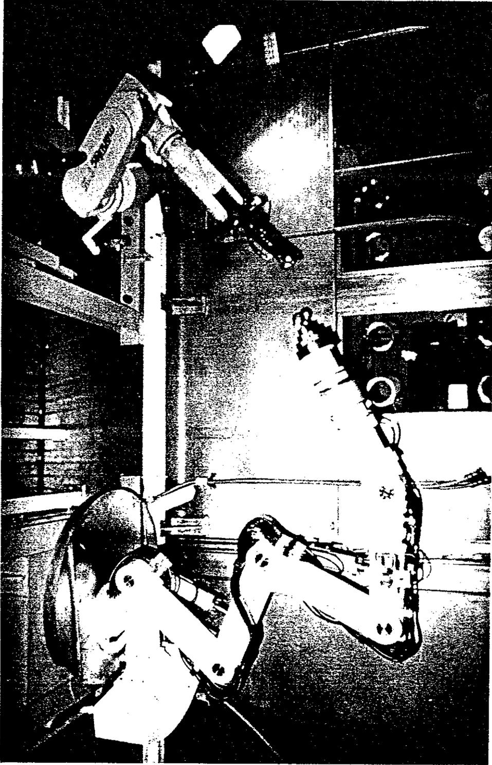
**Fig. 4.4 Power master - slave manipulator and plasma - torch
