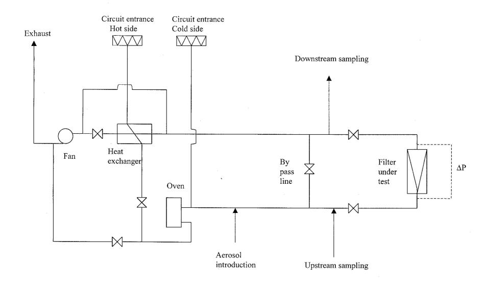
SIMOUN: A high temperature test loop
