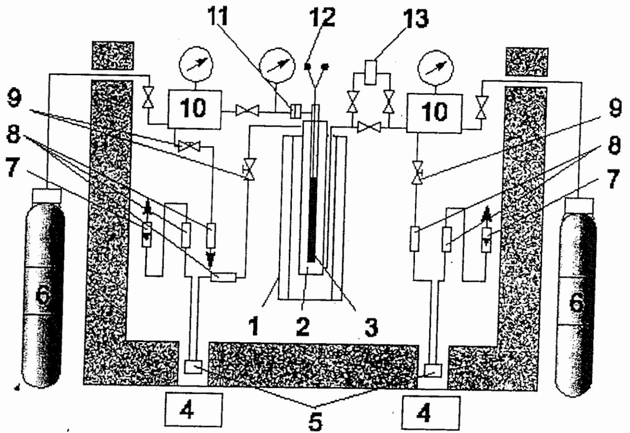
Fig.3. In-cell test rig for gas loading
