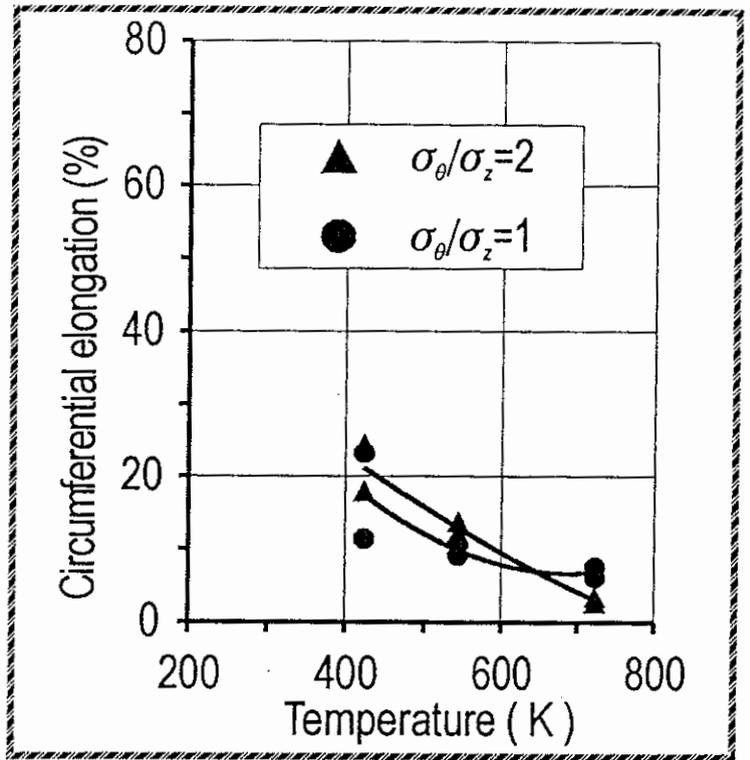
Fig.5 The influence of  $\sigma_\theta/\sigma_z$  relation on hoop strain of non-irradiated and irradiated VVER FE claddings
