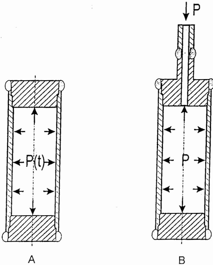
Fig.2. Samples for biaxial tension when  $\sigma_{\theta} / \sigma_z = 2$
