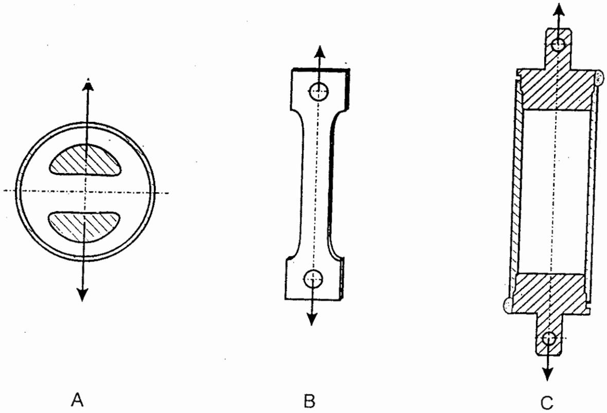
Fig.1. Samples for uniaxial tension
