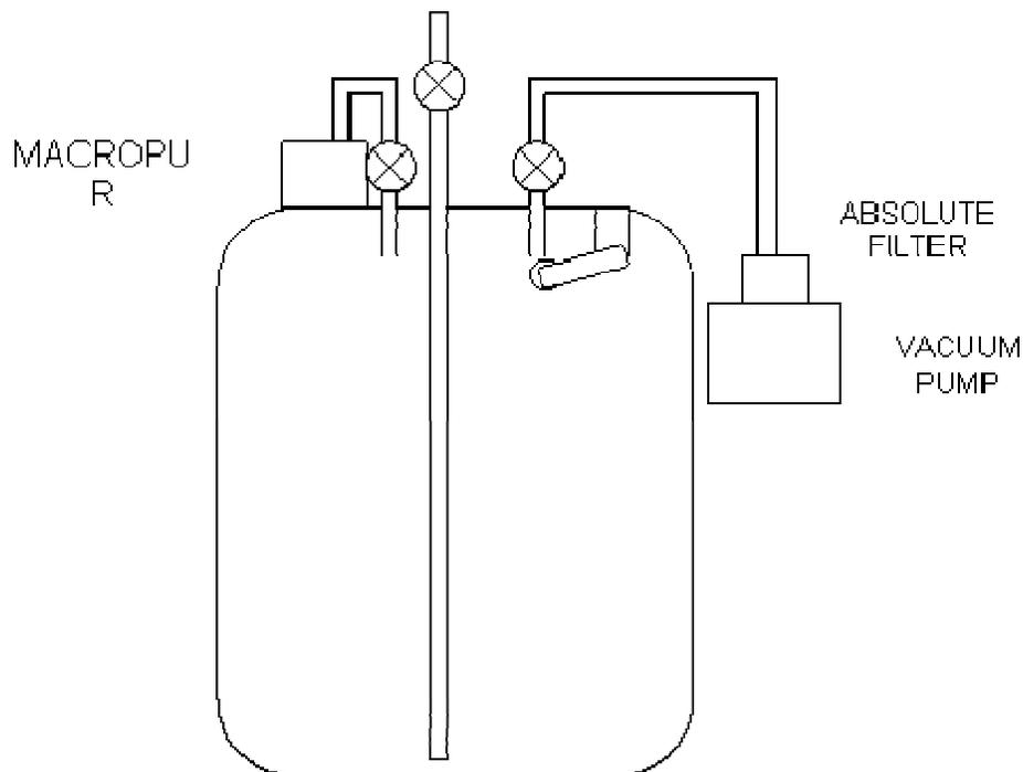
**FIGURE 4: conceptual chart of the connections from the cask to the Cendrillon loading system.**
