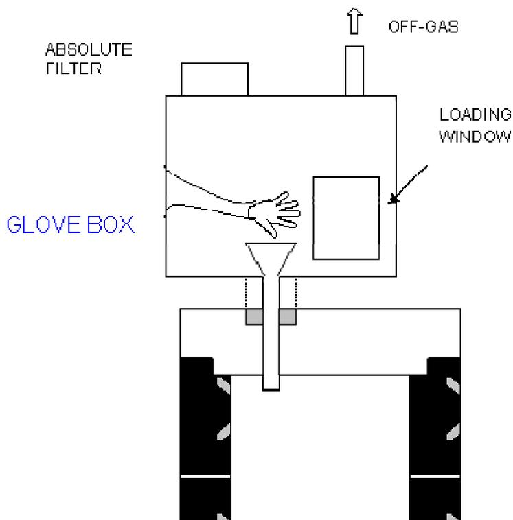
FIGURE 2: the manual load equipment arranged on the cask.
