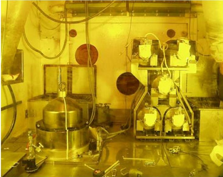
Figure 6: TIG welding device in K9 hot cell
