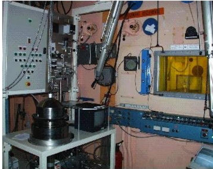
Figure 2: pressure vessel, with a movable hemispherical top cap, an immovable base and a nut
