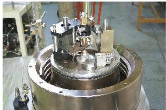
Figure 3 : the furnaces before their introduction in the hot cell
