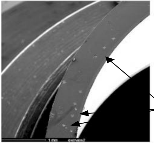
Fig.2 a: Positioning of the Vickers' indentation marks (arrows)
