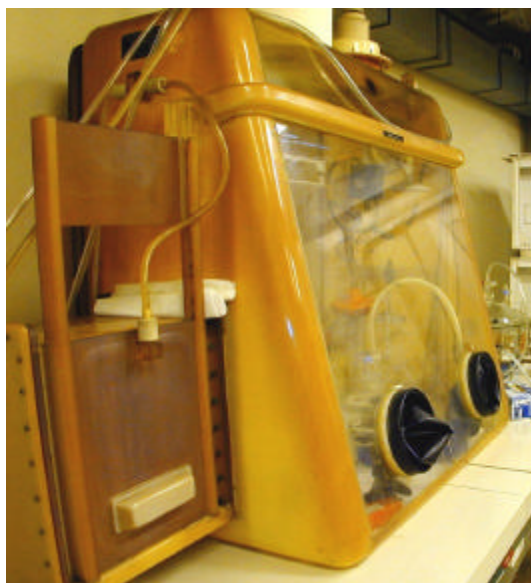
Figure 3. The anhydrous glove box for IR sample preparation.
