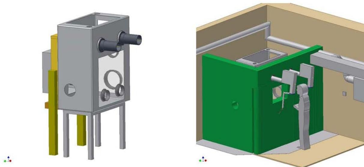
**Fig. 6** "Backpack"-solution for furnace being part of the  $\alpha$ -box, overview over the assembly
