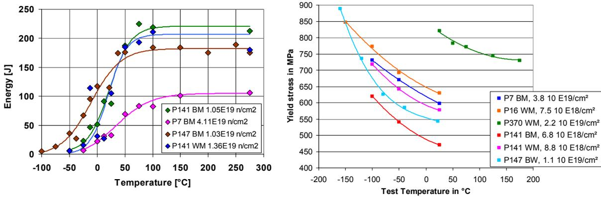
**Figure 3.** Results of the Charpy-V tests and the results of the yield stress versus test temperature curve of the tensile tests
