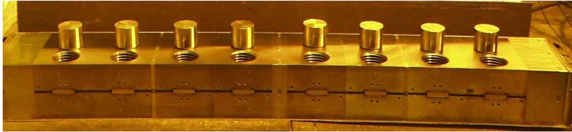
**Figure 2.** Opened capsule with a row of WOL-100X specimens.
