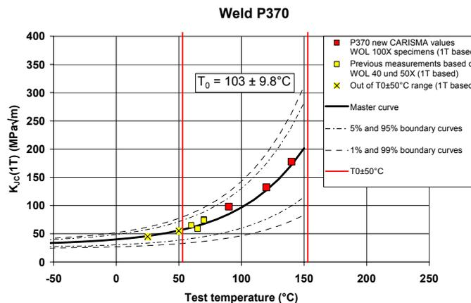
**Figure 4.** Fracture toughness curve of the irradiated weld material.
