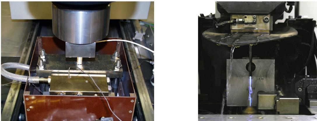
**Figure 6.** Test facility for CCA specimens and manufacturing of the side groove by EDM
