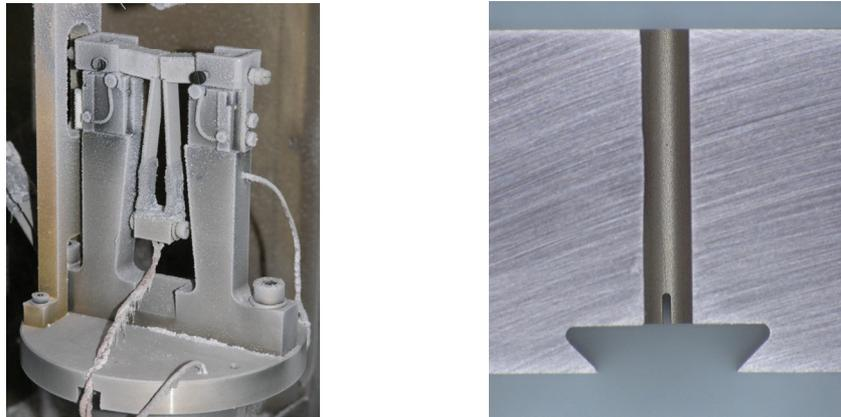
**Figure 5** Test facility for 10x10 SE(B) specimens and detail side view of a 10x10 SE(B) specimen
