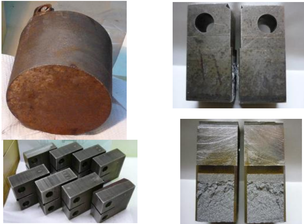
Fig.11. Steps of 1T-CT type specimens from 140 mm in diameter EPR RPV trepan manufacturing (left side) and testing.
