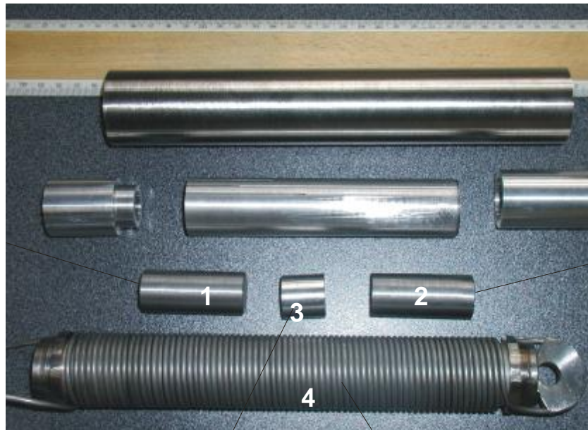
Fig.8. Experimental device for RPV steel billets irradiation. (1 and 2 – RPV metal billets, 3 - capsule for neutron monitors, 4 – heater)
