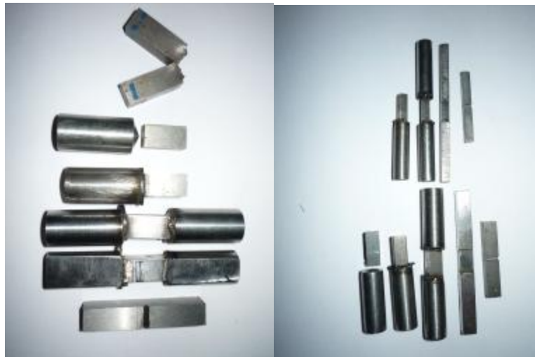
Fig.6. Examples of the reconstitution technique application (arc stud welding) for materials recycling. Left: standard Charpy 10×10mm 2 ; .right: subsized Charpies 5×5mm 2 and 3×4mm 2 .
