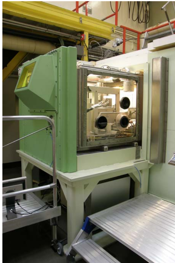
FIG. 3.3. Hot-cell with SEM. One lead wall and the roof is removed to show the equipment.
