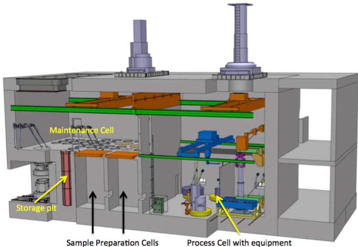
**Figure 3: Layout of the active cells that include the process cell and the sample preparation cells (figure credit: P. Erterius).**
