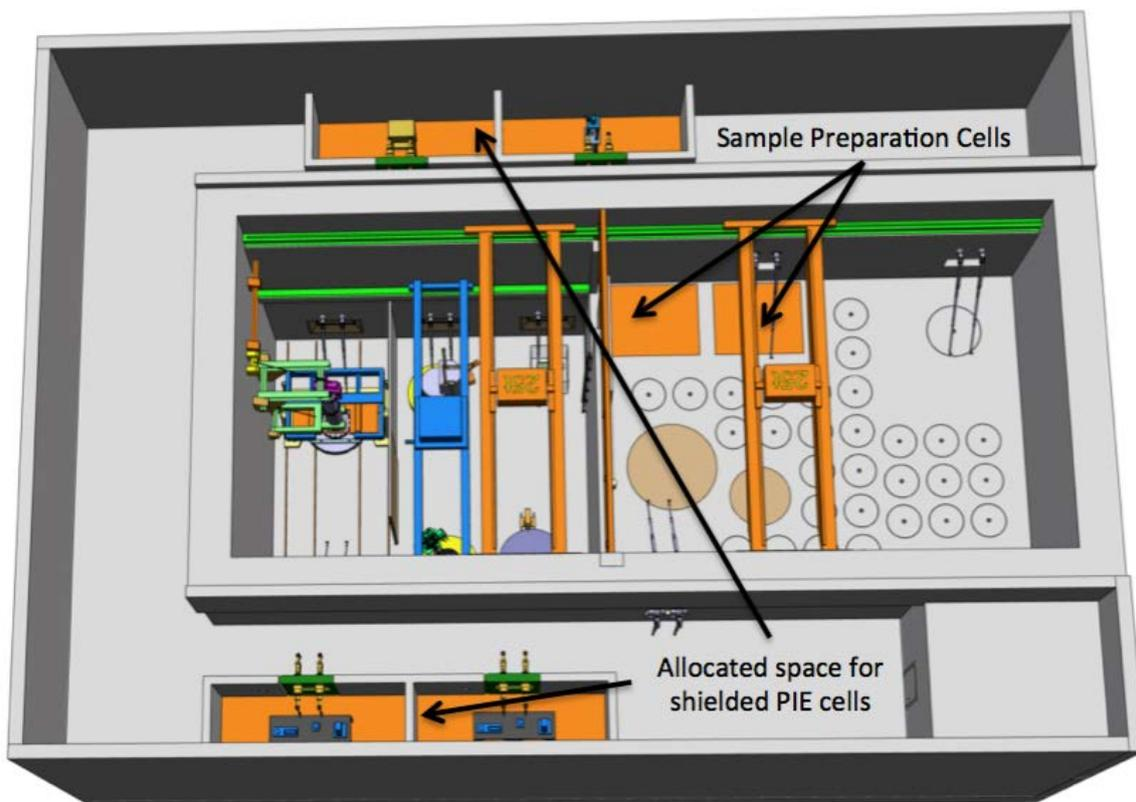
Figure 4: The space allocated for the shielded PIE Cells on the ground floor of the target building (figure credit: P. Erterius).
