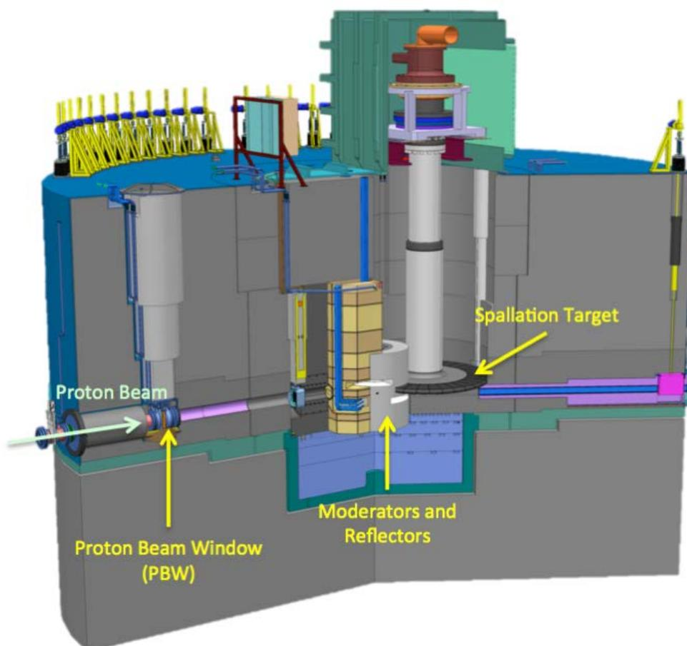
**Figure 1: Layout of the ESS Target Monolith that houses the spallation target, moderators, reflectors and proton beam window (figure credit: N. de la Cour).**
