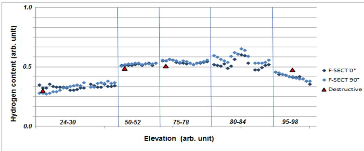
Fig. 8: Correlation between estimated electrical conductivity (blue point) and hydrogen content from destructive analysis (red points).
