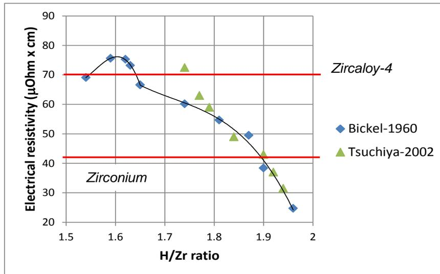
Fig. 2: Literature data on the electrical conductivity of Zr hydrides [5,6] compared to that of Zircaloy-4 .
