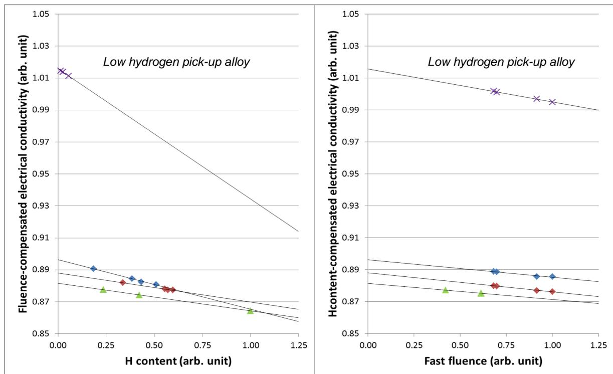
Fig. 9: Separation of the effects due to hydrogen absorption and fast neutron fluence on the electrical conductivity of different Zr-alloys.
