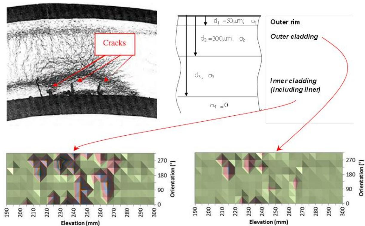
Fig. 10: Model used to analyse F-SECT data from fuel rods affected by secondary degradation, and color-coded maps of the electrical conductivity of the inner and outer parts of the cladding.
