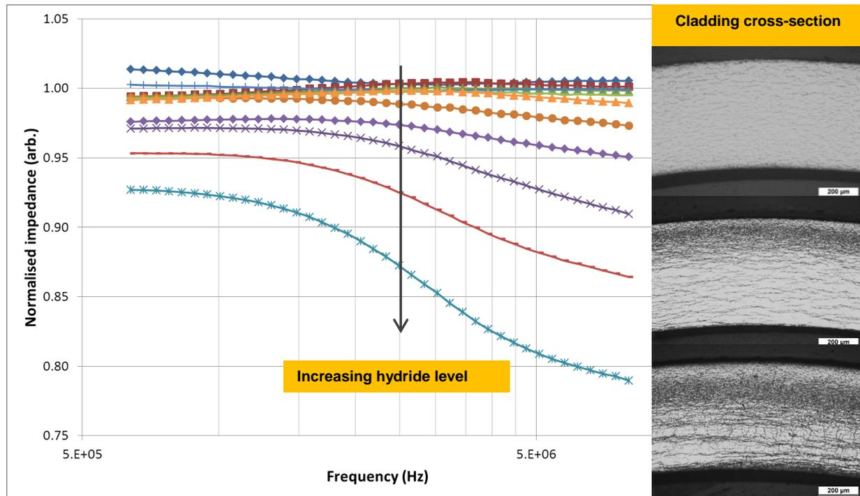
Fig. 1: Correlation between measured normalized impedance vs. frequency curves and cladding condition.
