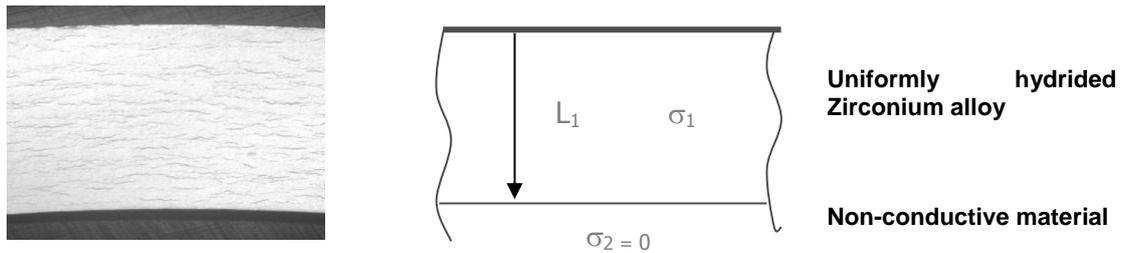
Fig. 4: 2-layer model for uniformly hydrided zirconium alloy.
