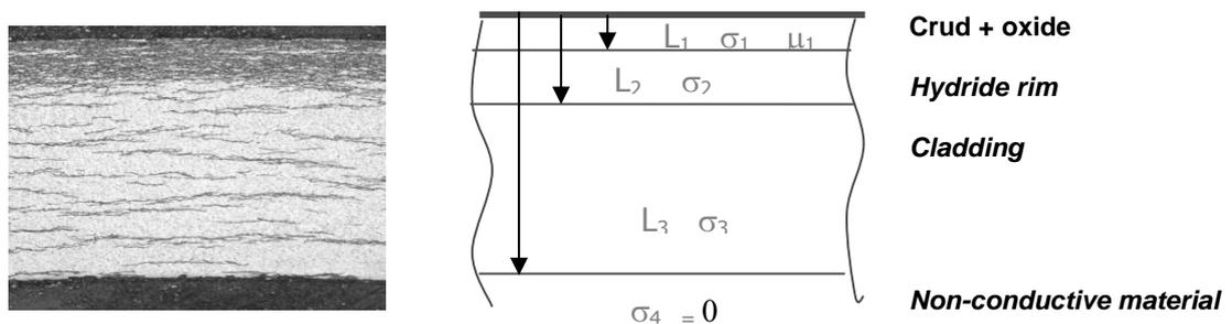
Fig. 6: 4-layer model for zirconium alloy with hydride rim and ferromagnetic deposits (crud).
