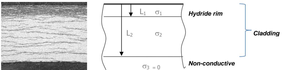
Fig. 5: 3-layer model for zirconium alloy with a hydride rim.
