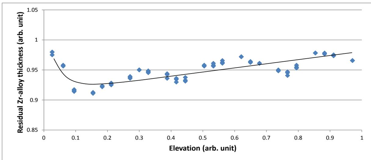
Fig. 7b: Example of residual Zr-alloy thickness measured on the same rod of figure 7a.
