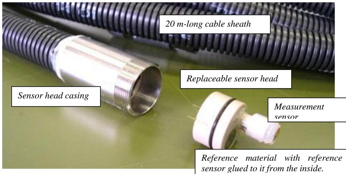
Fig. 3: 20-meter long, water-tight connection cable and replaceable self-nulling sensor.
