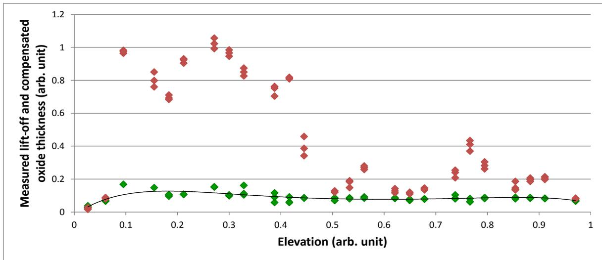
Fig. 7a: Measured (red) and compensated (green) oxide + crud thickness on a fuel rod.
