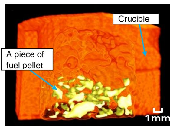
**Figure 4** Three-dimensional X-ray CT image of simulated fuel debris specimen
