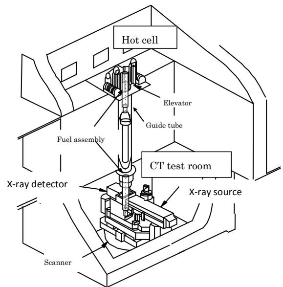
Figure 1 Outline of X-ray CT apparatus
