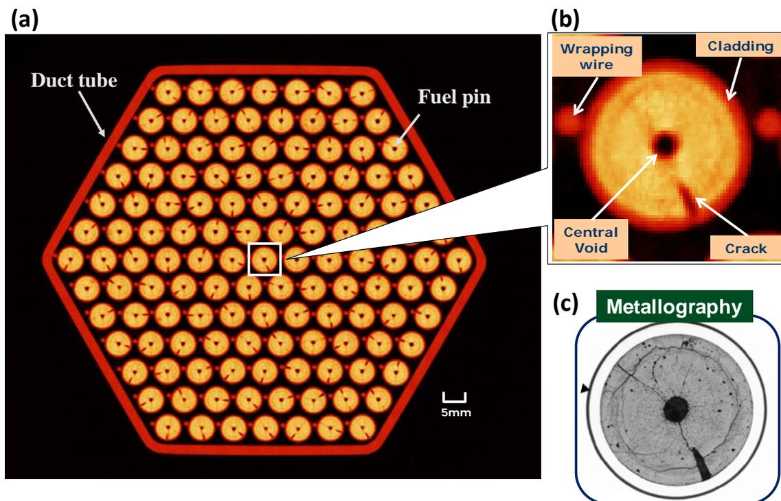
**Figure 3** Cross-sectional X-ray CT images obtained from the irradiated fuel assembly
