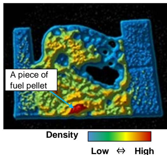
**Figure 5** Density distribution obtained by analyzing X-ray CT image
