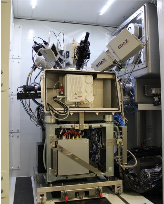
Secondary electrons (SE) are detected with an Everhart-Thornley-type chamber detector and with the in-lens SE-detector. For the detection of Back-Scattered Electrons (BSE) a YAG-detector and an in-lens EsB (Energy selective Backscatter) will be available.
