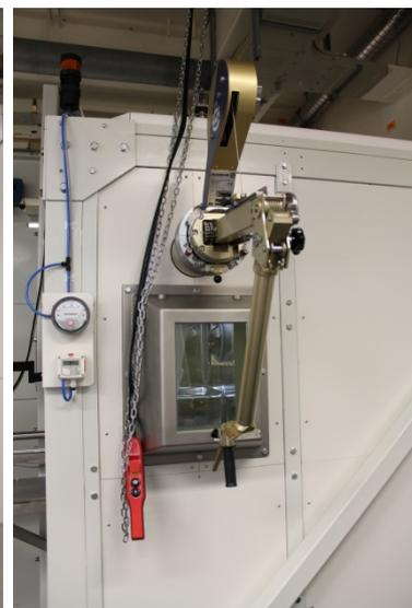
Fig. 4: lead glass window and tele-manipulator
