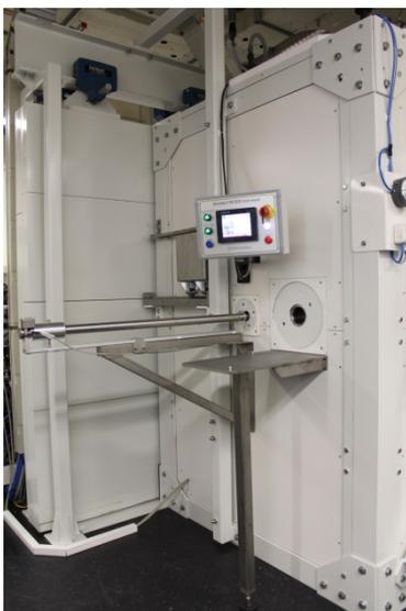
Fig. 2: Hot Cell with transfer systems
