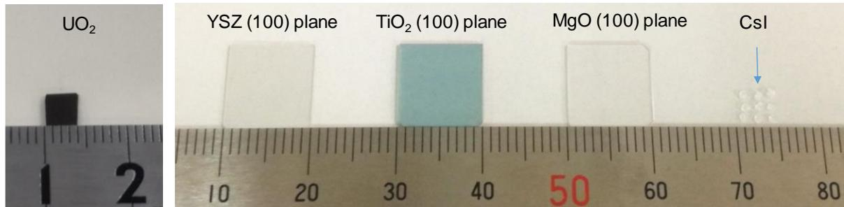
Fig. 1. Appearances of the samples used for the sessile drop test.
