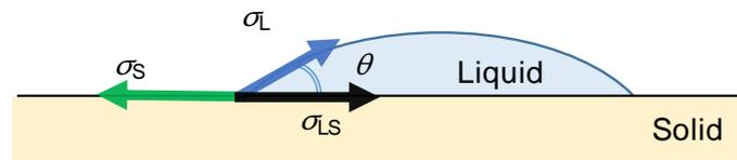
Fig. 2. Schematic image of the sessile drop test and the balance of Young's equation.
