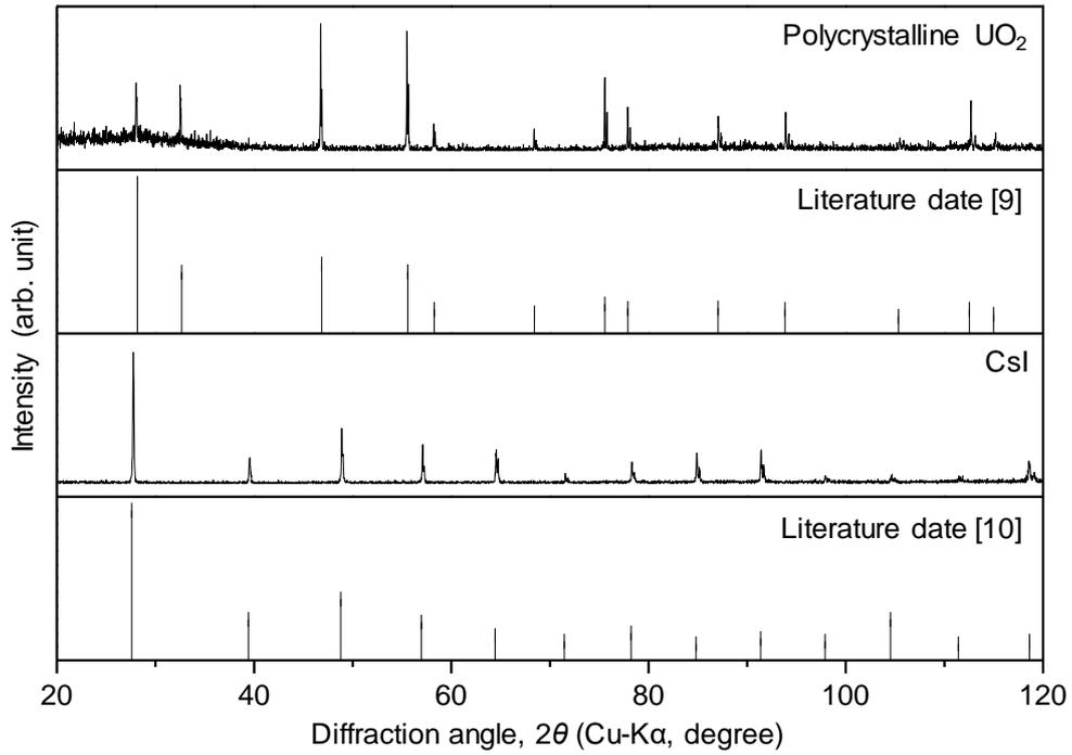
Fig. 3. XRD patterns of polycrystalline UO<sub>2</sub> and CsI used for the sessile drop test.
