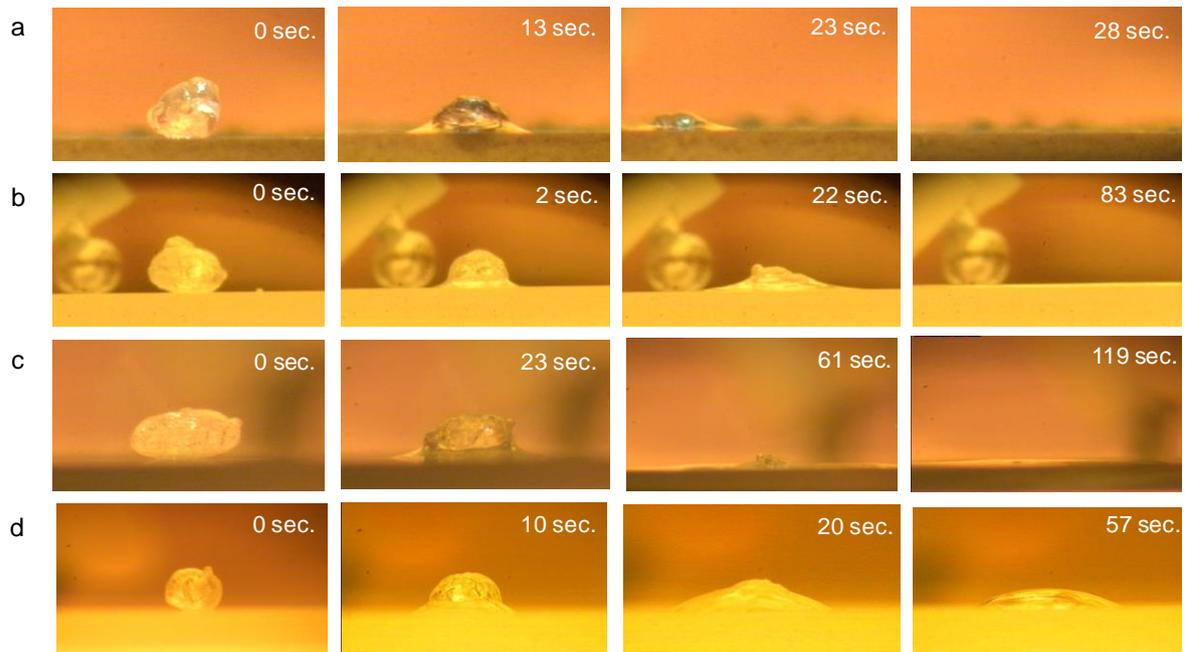
Fig. 5. Melting behaviour of CsI on various solid samples. (a) polycrystalline  $\text{UO}_2$ , (b) YSZ (100) plane, (c)  $\text{TiO}_2$  (100) plane, and (d) MgO (100) plane.
