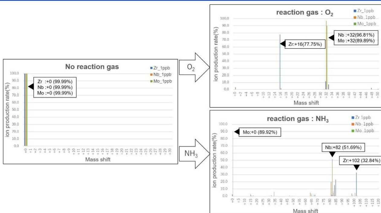
Figure 36: Ion production rate (Mass spectra) of QQQ- ICP -MS
