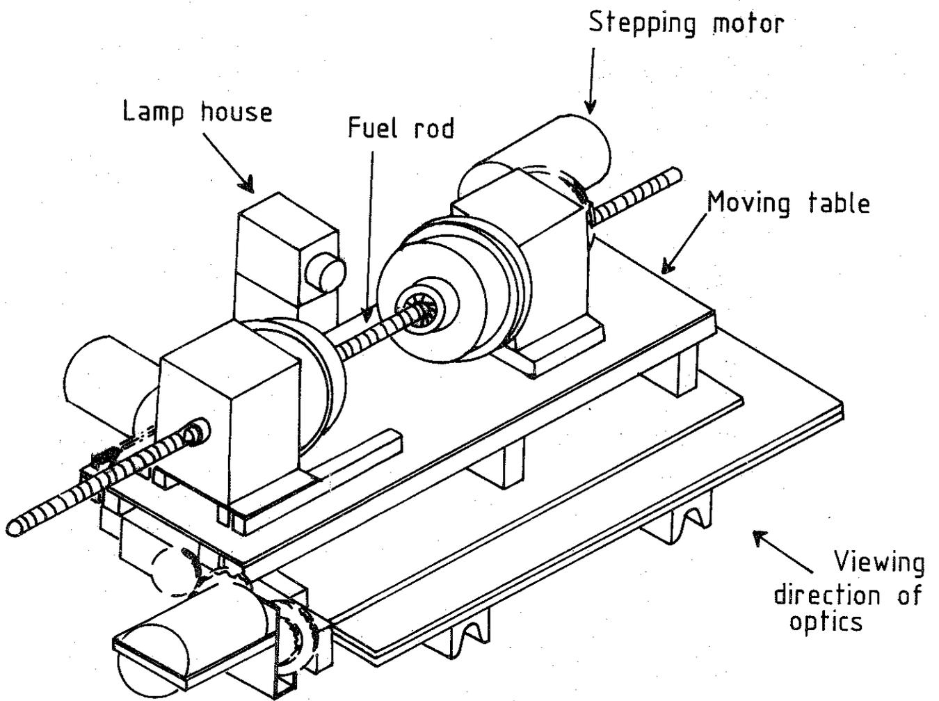
FIG. 9 IN-CAVE PIN HANDLING RIG
