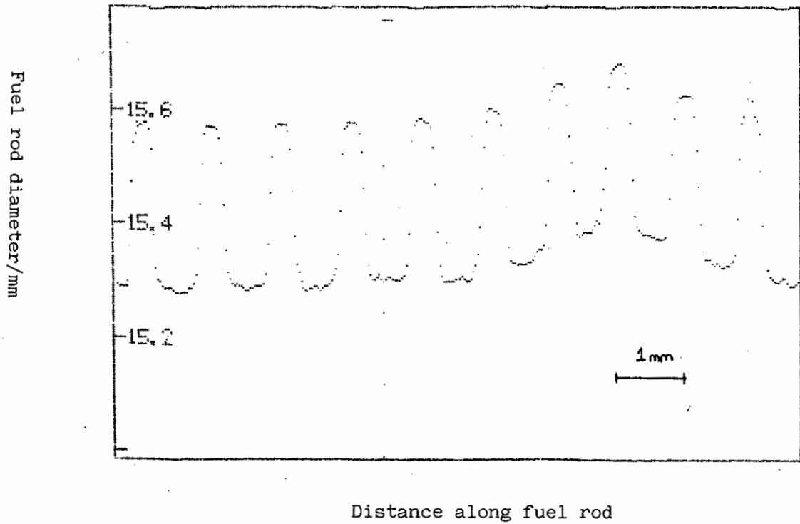
FIG 8 PRINT-OUT OF A COMPUTER GRAPHICS DISPLAY SHOWING THE DIAMETRAL VARIATIONS ALONG A SECTION OF UNIRRADIATED AGR FUEL ROD
