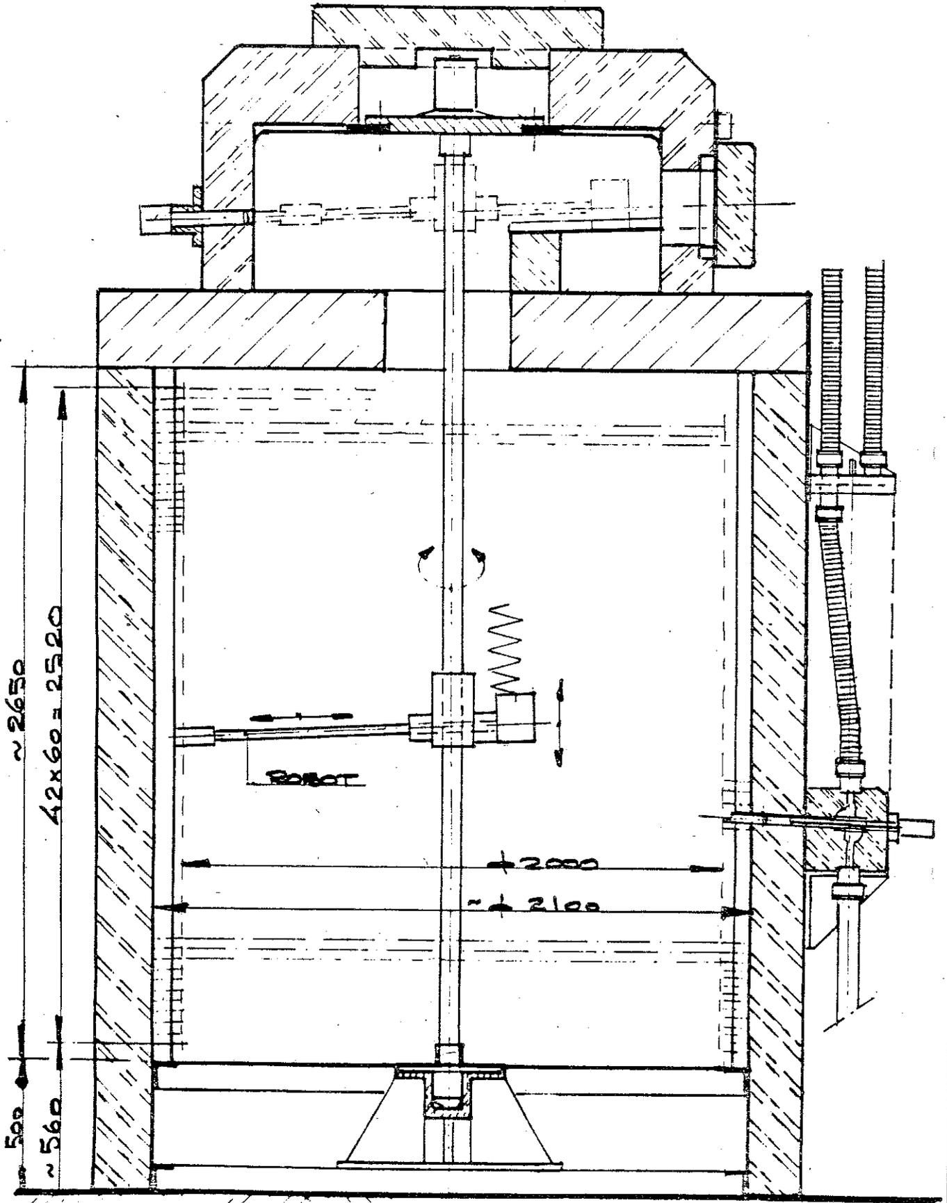
Figure 1. Cross section of a direct access store with simple robot arm
