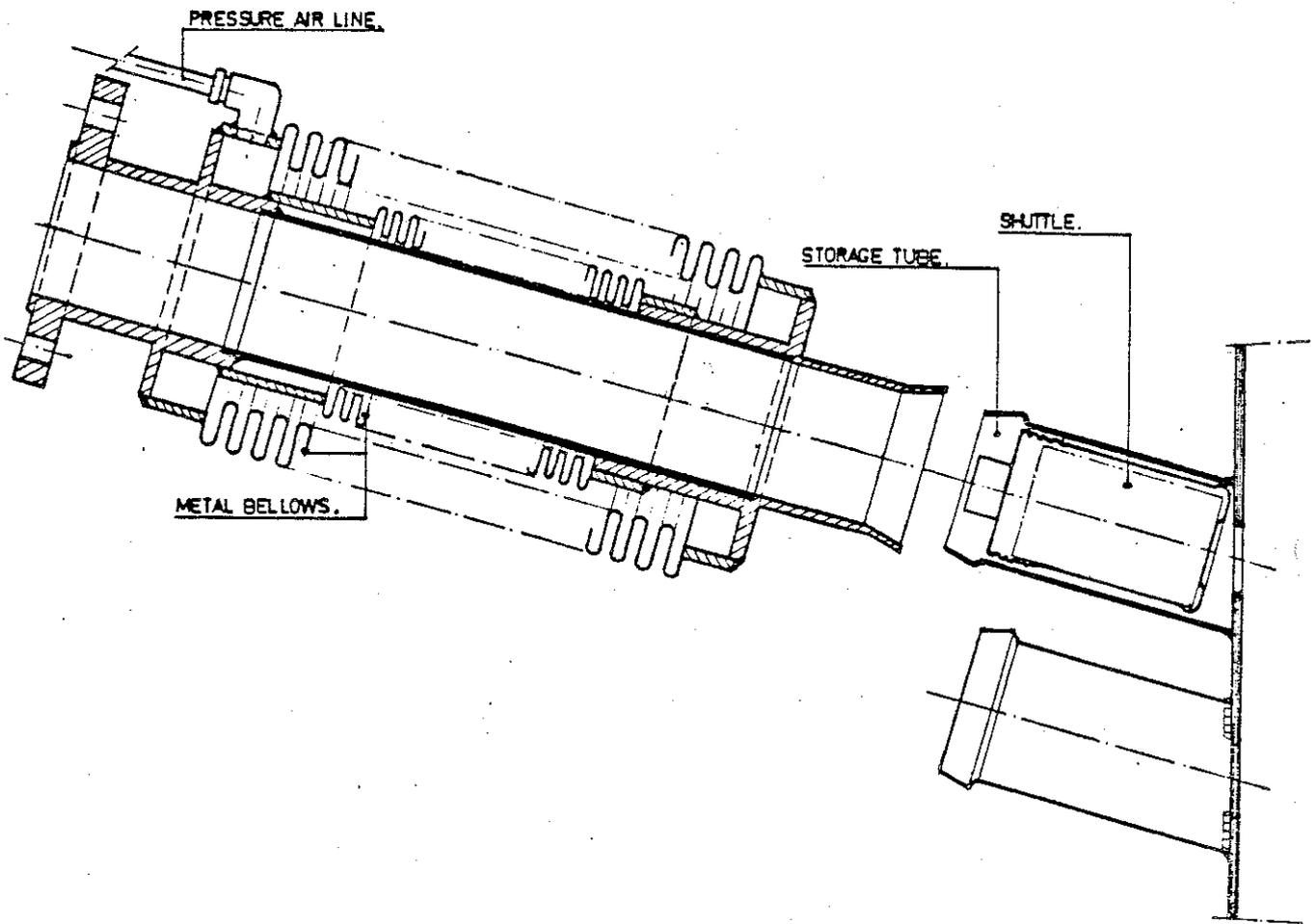
Figure 3. Detail of charge/discharge bellows assembly of alternative design
