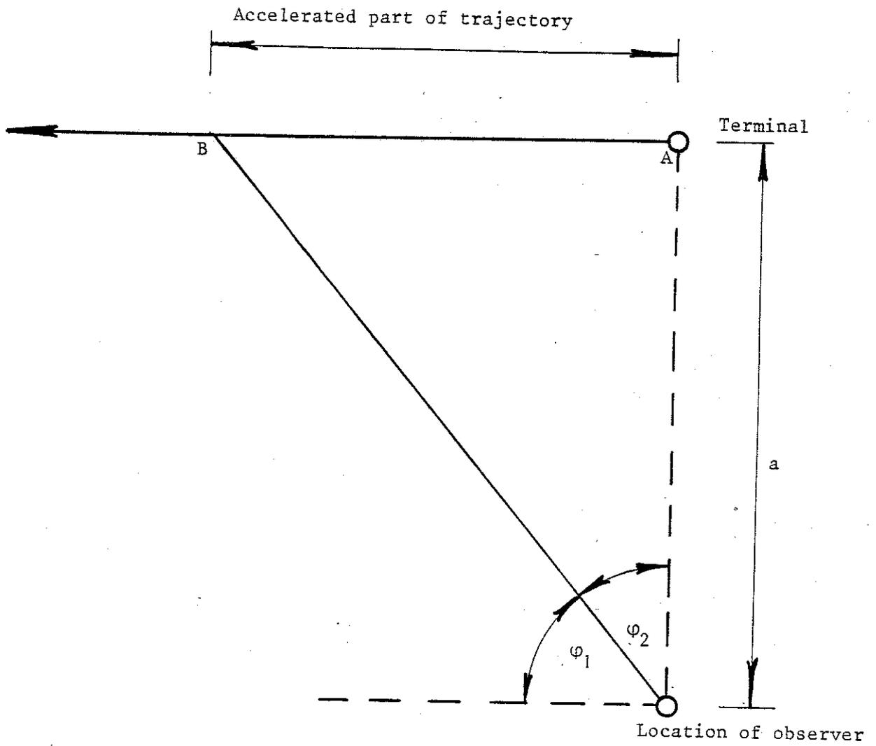
Shuttle departing from terminal A with velocity = 0 has reached velocity of  $V_0$  cm/sec at point B.
