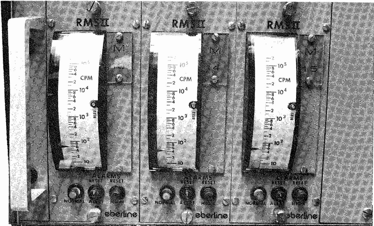
Fig. 3.5. Five decade rate meters of the 2-of-3 system.
