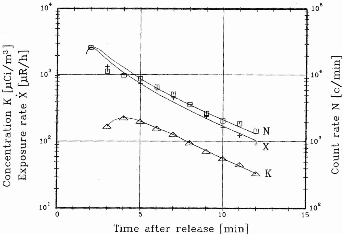
Fig. 4.1. Measured count rate (N) from the iodine/particular monitors, exposure rate ( $\dot{X}$ ) from the GM-system and concentration (K) in the ventilation channel after a momentary release of 1.5 Ci  $^{41}\text{Ar}$ . Unshielded 2-of-3 monitors.
