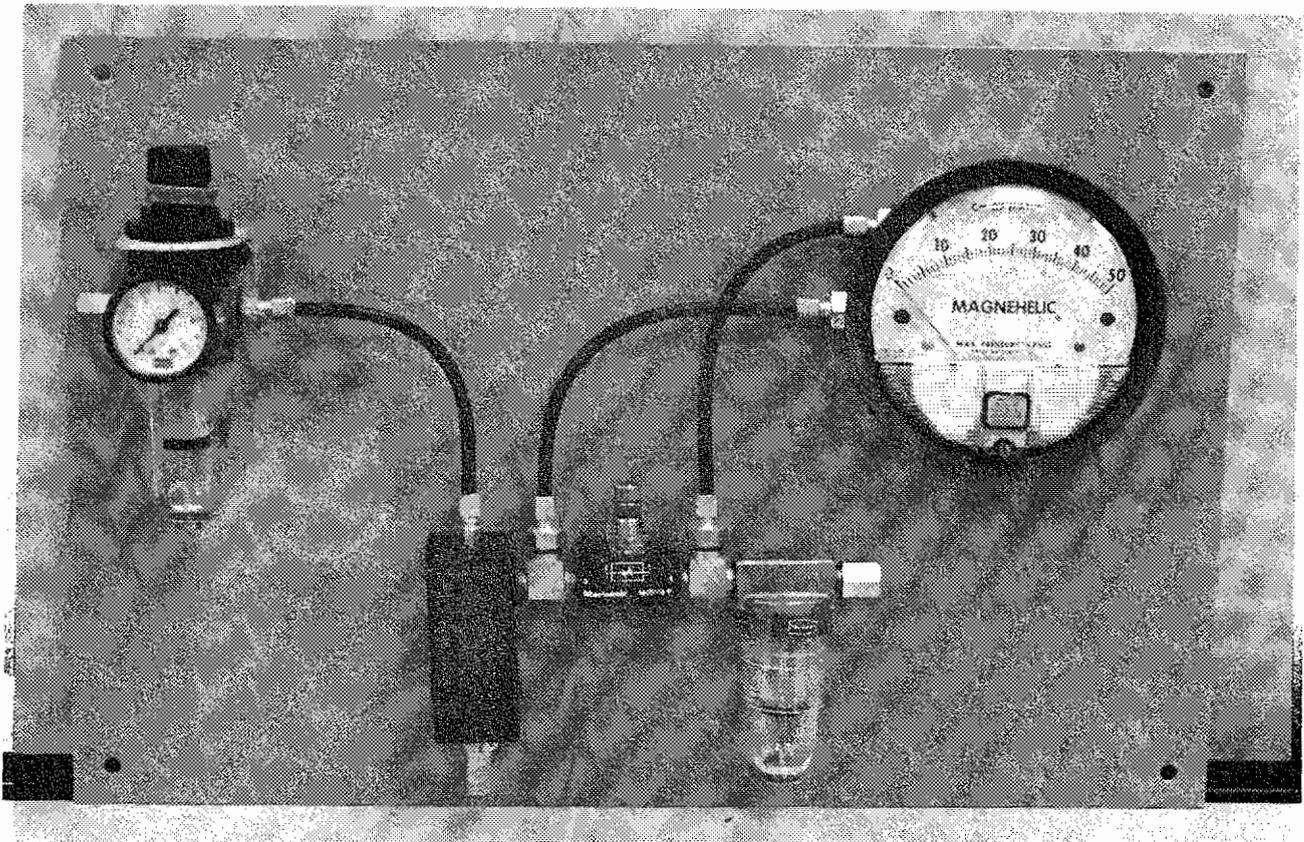
Fig. 3.4. Air ejector arrangement with air flow controllers.
