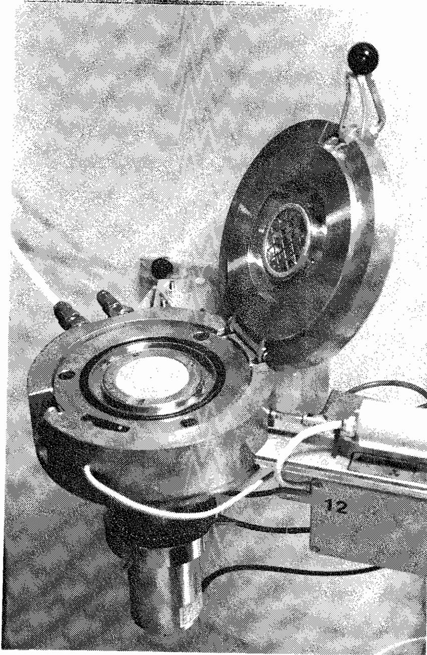
Fig. 3.2. Air flow house with detector, filter papers, and check source facility.
