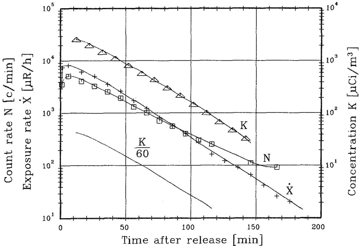
Fig. 4.2. Measured count rate (N) from the iodine/particular monitors, exposure rate (X) from the GM-system, and concentration (K) in the ventilation channel for recirculation and concentration  $K/60$  in the ventilation channel after a momentary release of 1.5 Ci  $^{41}\text{Ar}$ . Lead shield of 2 cm around the flow house.
