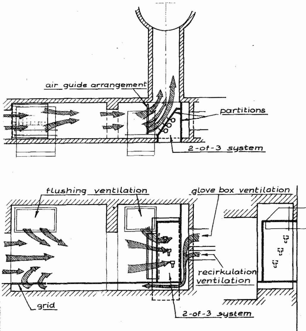
Fig. 2.1. The ventilation outlet with the 2-of-3 system.
