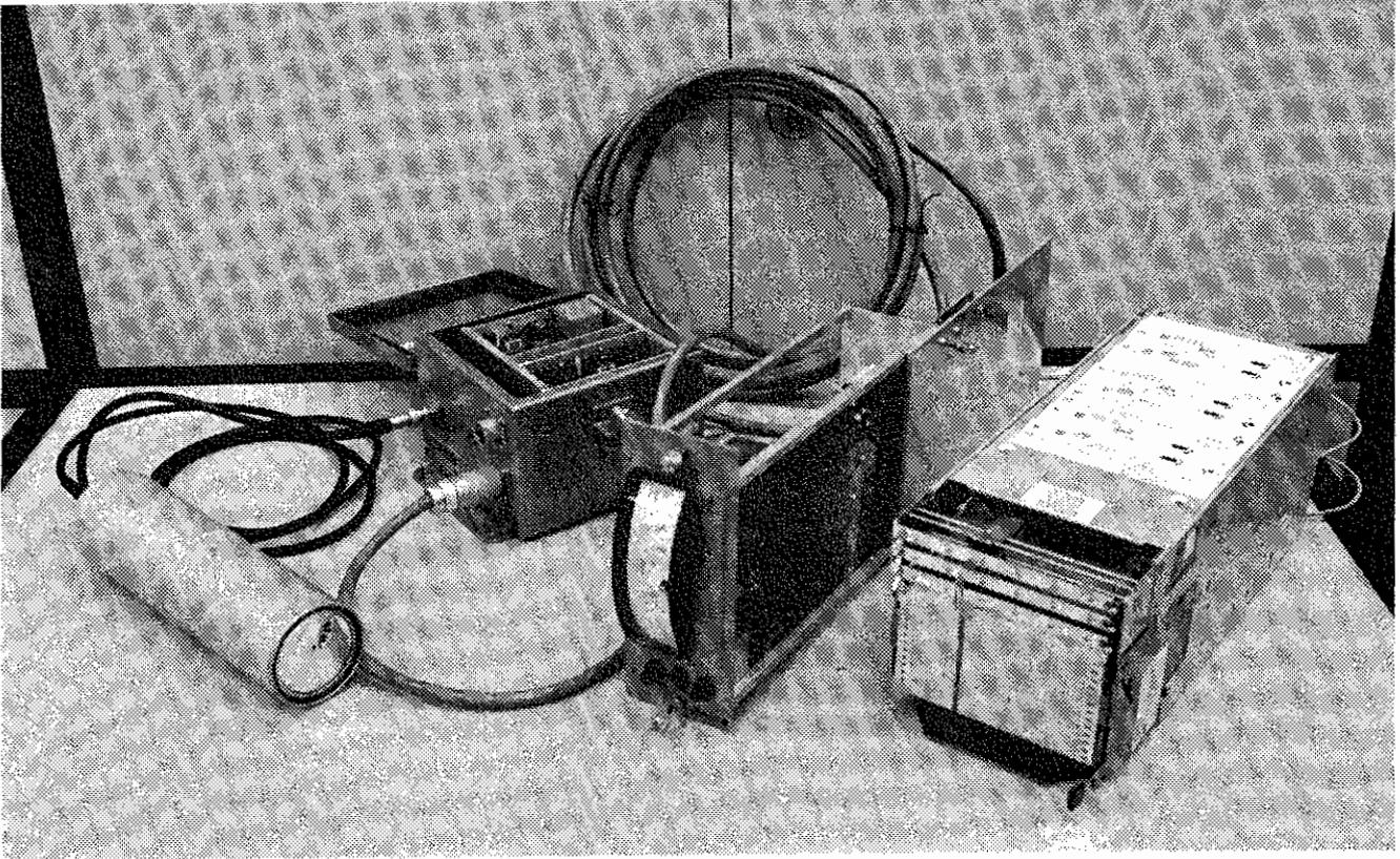
Fig. 3.1. Beta detector, interface/power supply, rate meter and recorder.
