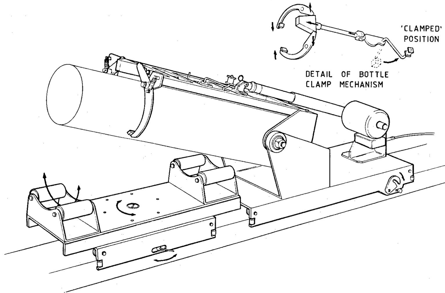
FIG.5 CAGR FUEL ELEMENT TILTING BUCKET AND CRADLE
