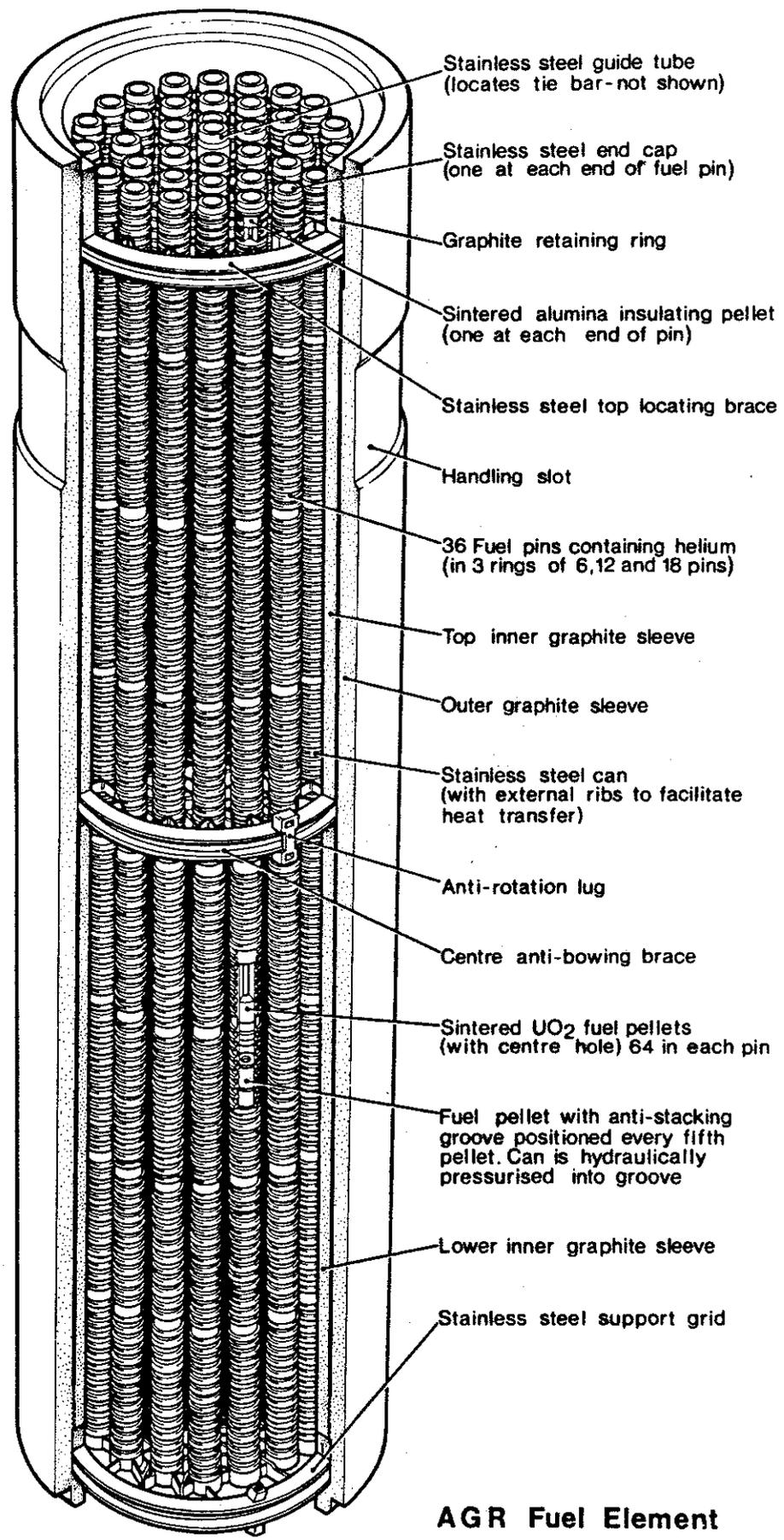
Fig. 2 Cut-away Diagram of the CAGR Fuel Element.
