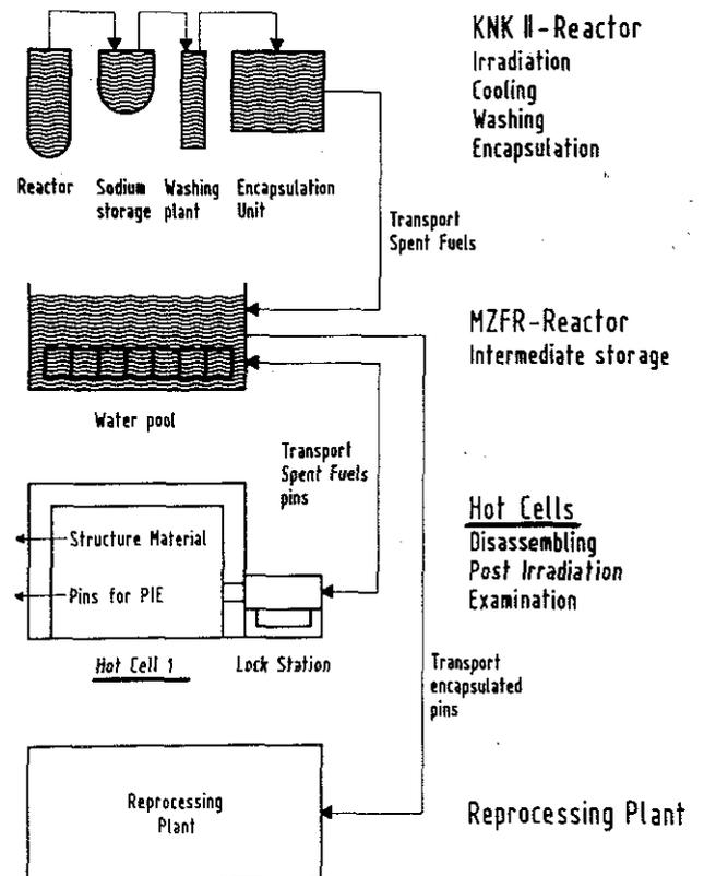
Fig. 5 The role of the Hot Cells in the disposal of the KNK II fuel elements.
