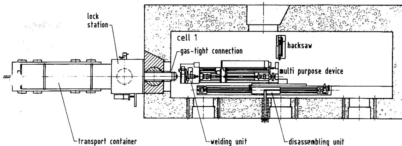
Fig. 6 Arrangement of the four large devices for transfer, measurement, disassembly and welding in cell no. 1.
