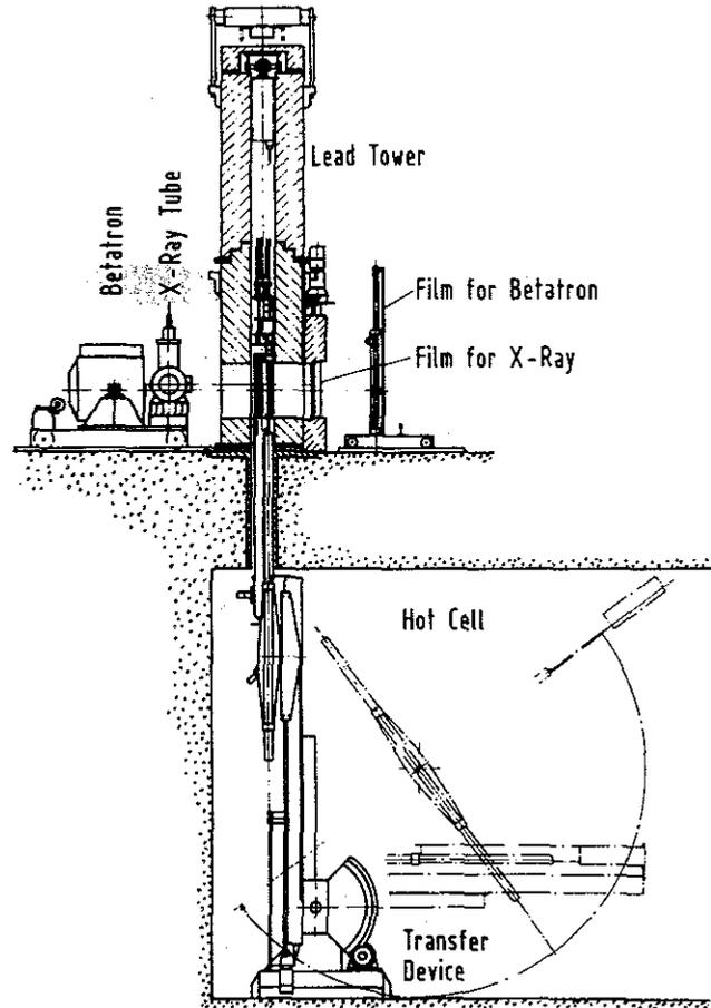
Fig. 3 Arrangement of lead shielded tower, X-ray or betatron and film holding device above the cell, pin transfer device in the cell.
