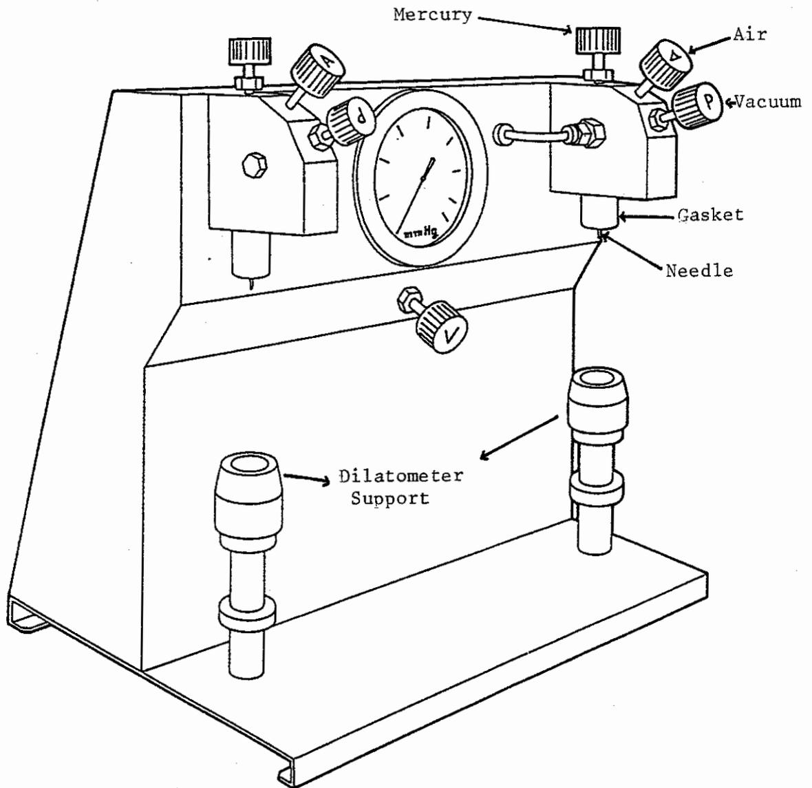
Fig.2 : Duplex dilatometer filling unit
