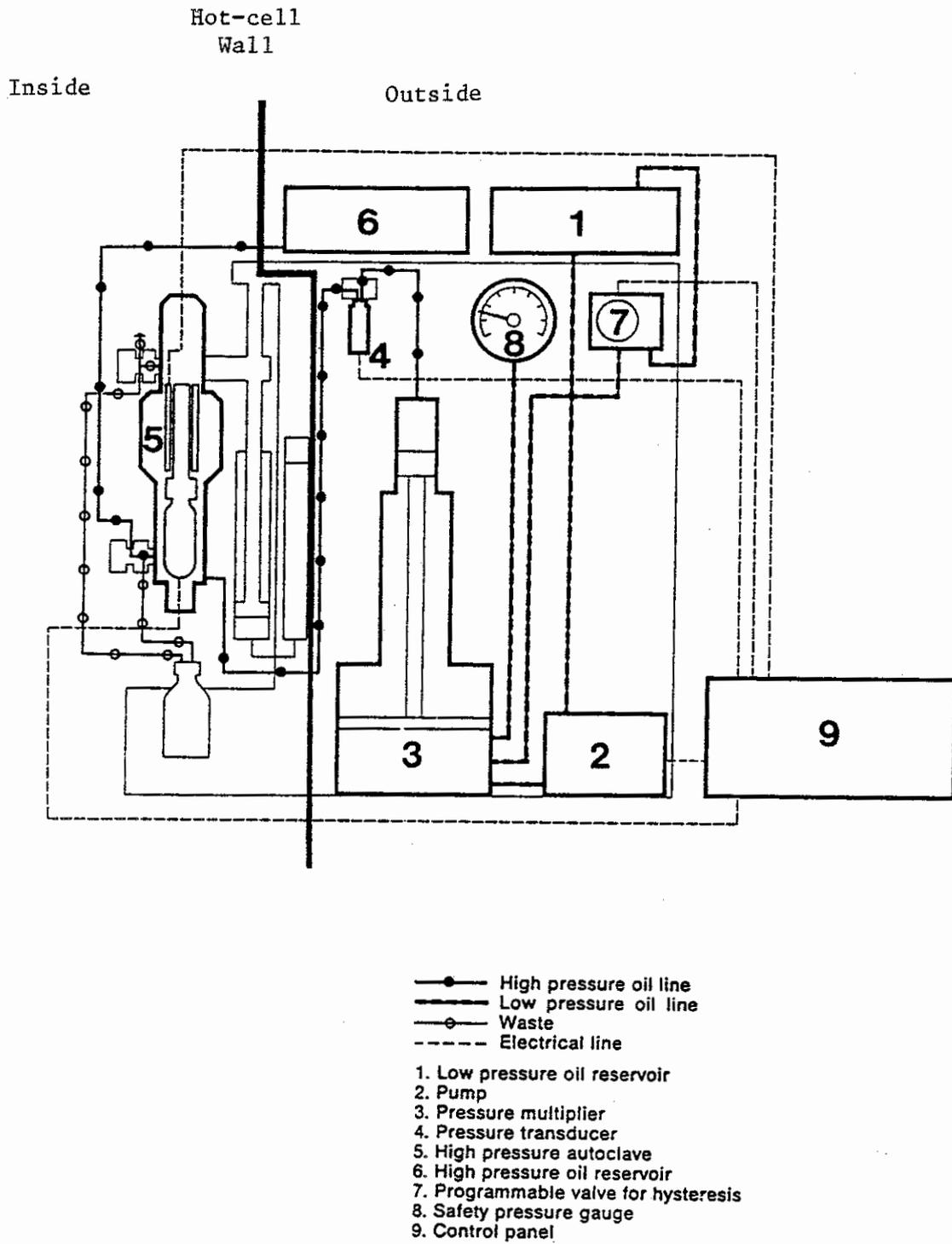
Fig. 4 : Schematic performance of the Analytical Unit
