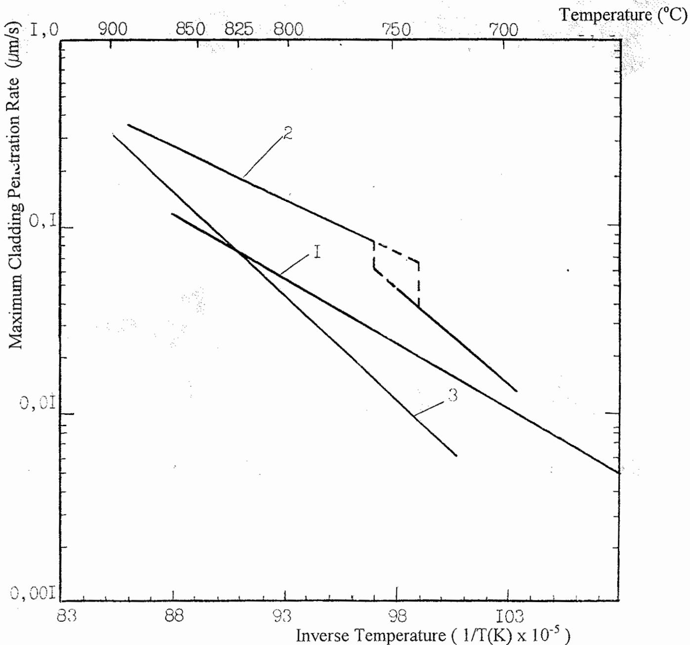
Fig.5. Cladding penetration rate vs temperature for 1-h tests
