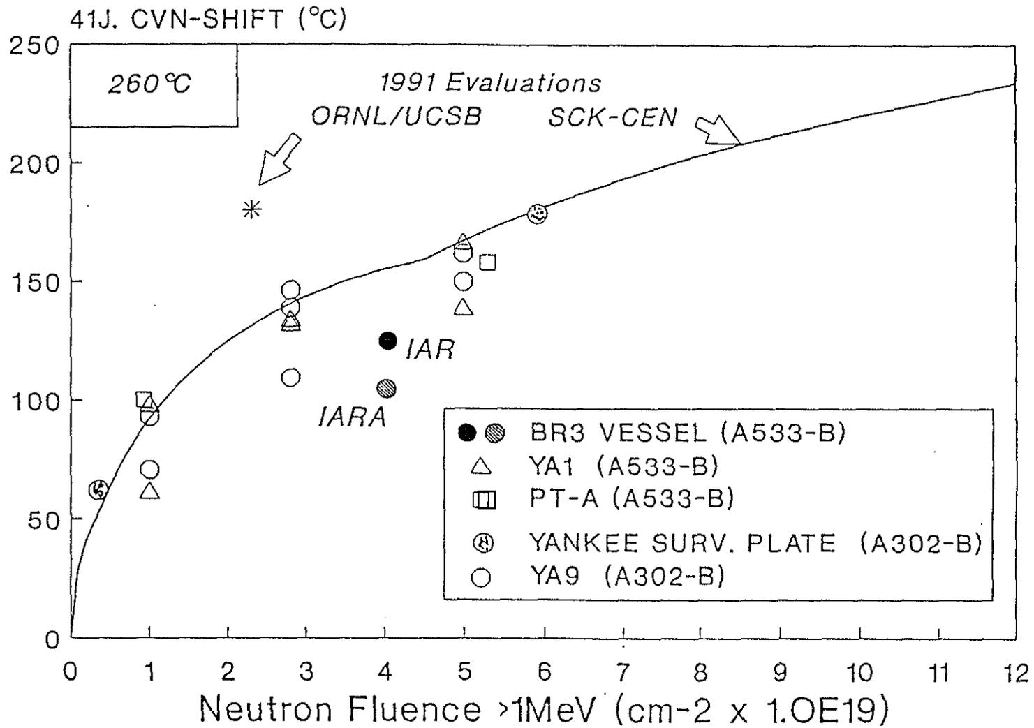
FIGURE 3 The BR3 plate embrittlement is less than predicted and lack of Ni influence is confirmed
