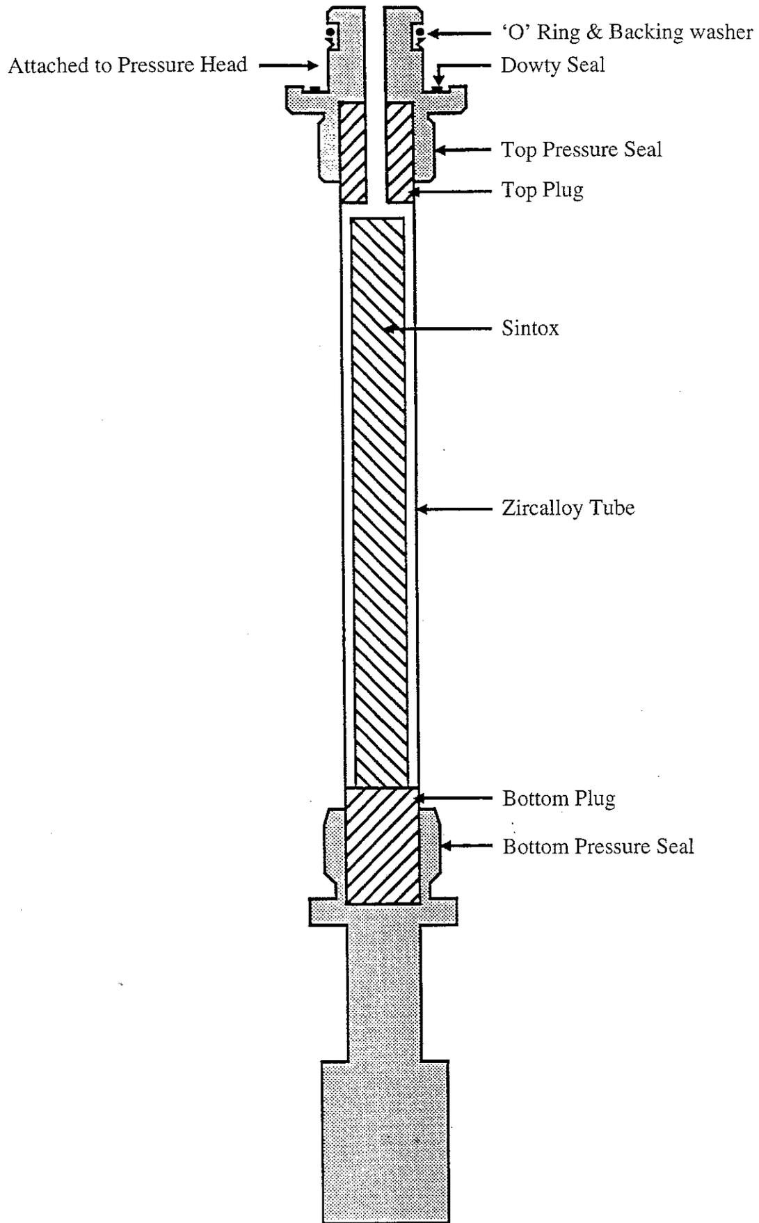
Figure 3: Specimen Design.
