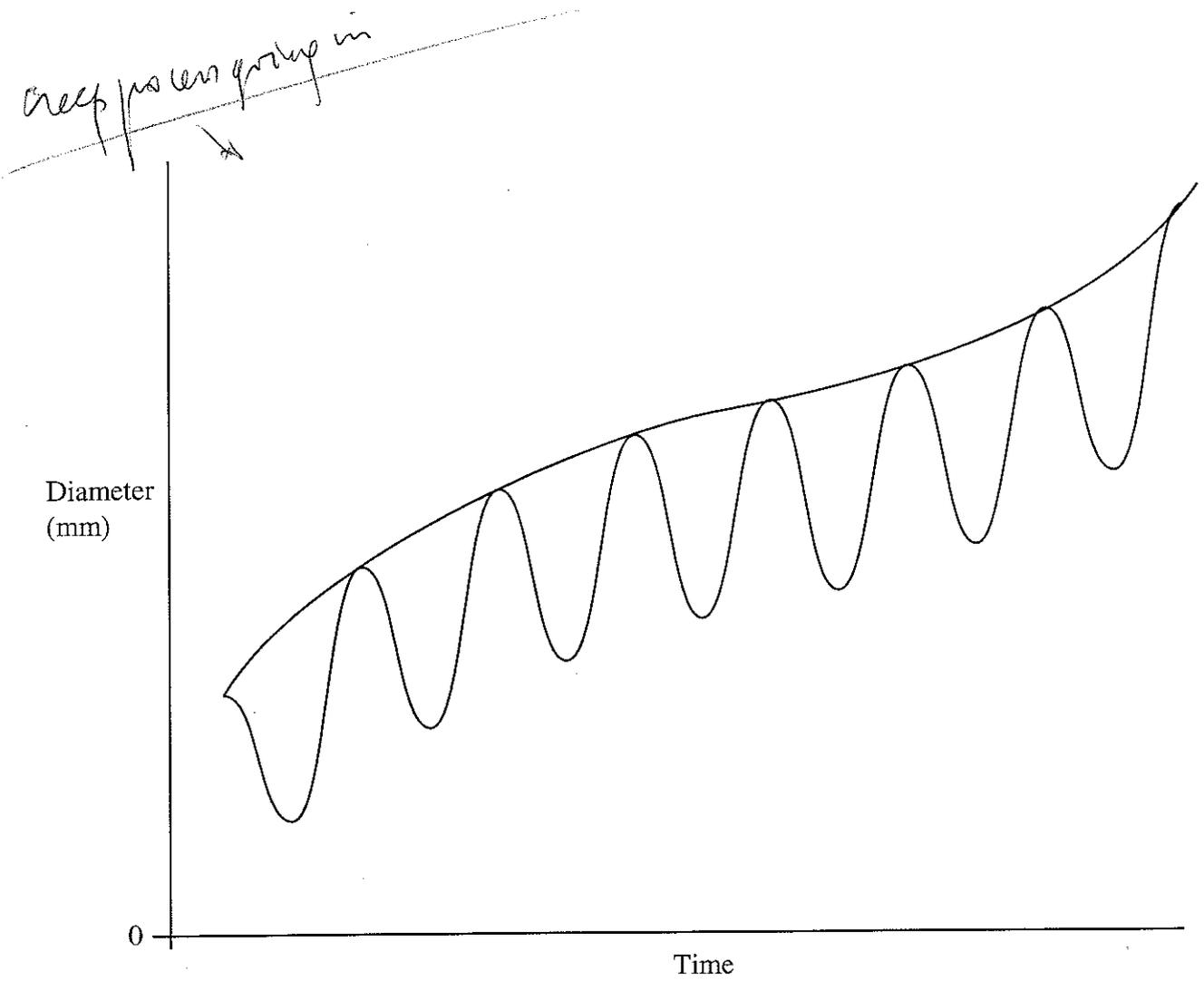
Figure 5: Schematic LCF Test Record.
