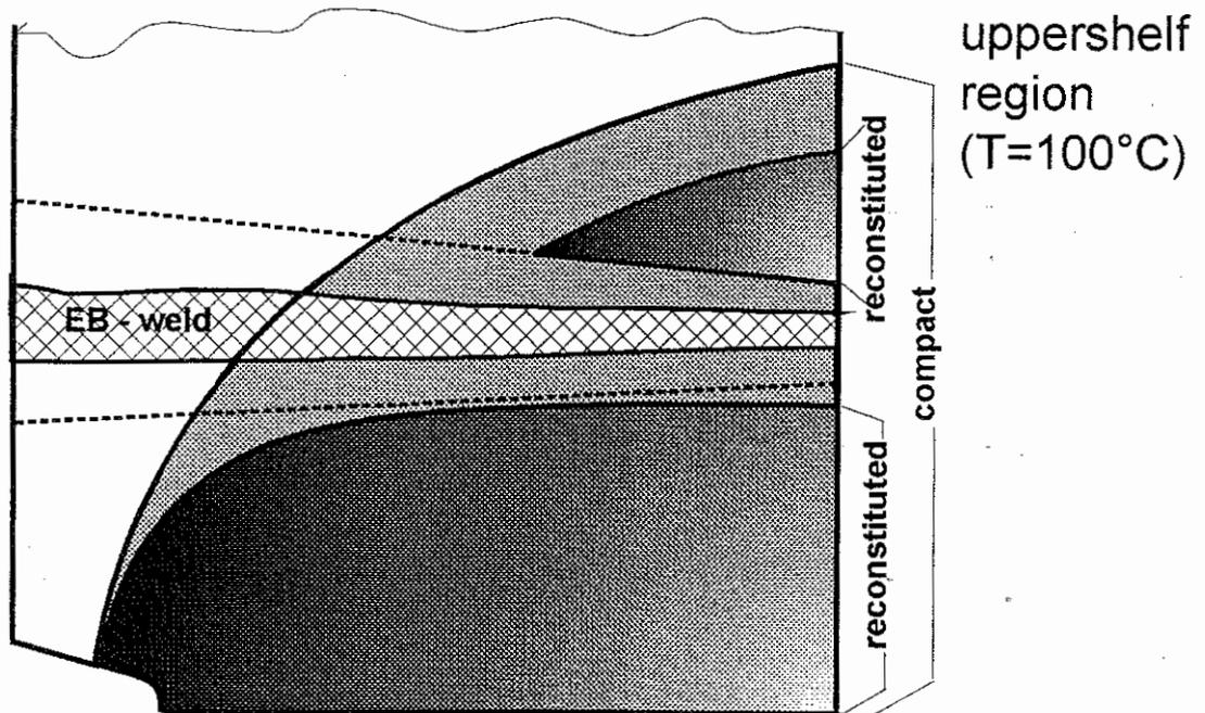
Comparison of the Plastic Zones of Compact and Reconstituted Specimens measured by Hardness
