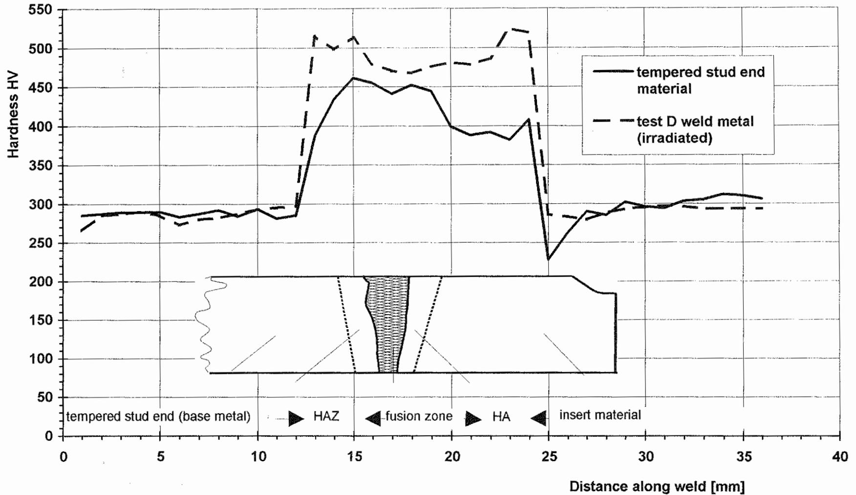
**Hardness Distribution after EB Welding, Weld Metal (irradiated condition)**
