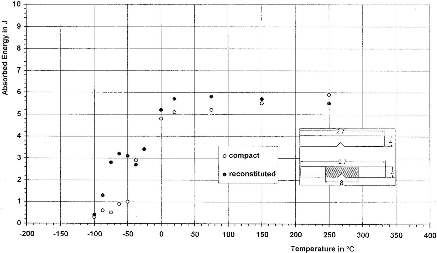
Charpy Energy of Mini Charpy Specimens, Weld Metal (non-irradiated condition)
