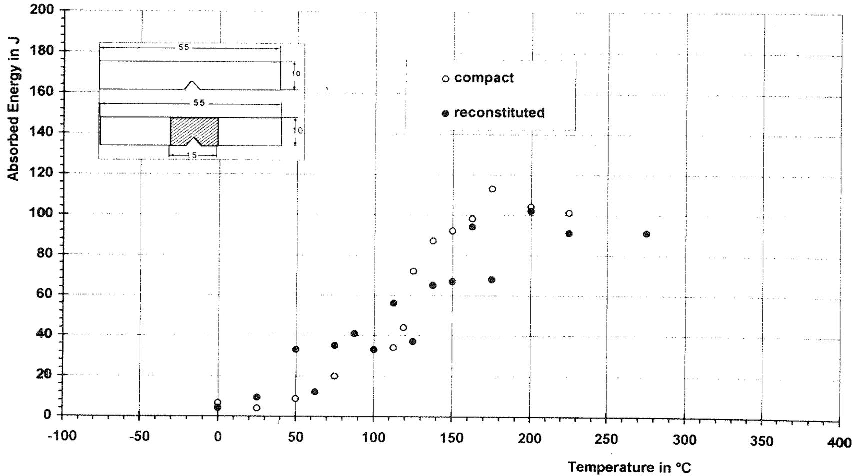
**Charpy Energy of Normal Size Specimens, Weld Metal (irradiated condition)**
