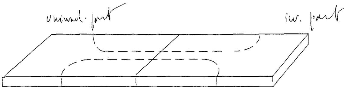
Figure 5 Schematic of butt-welded joint and projected flat tensile specimen.
