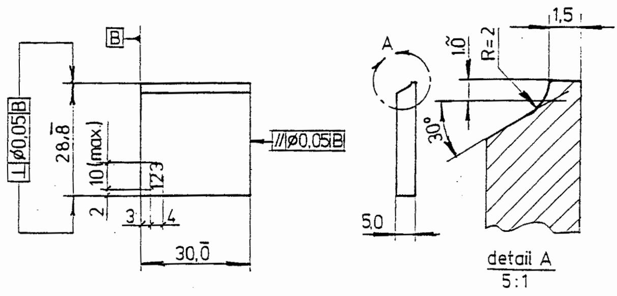
Figure 6 Dimensions of Y-type groove for 5 mm samples.
