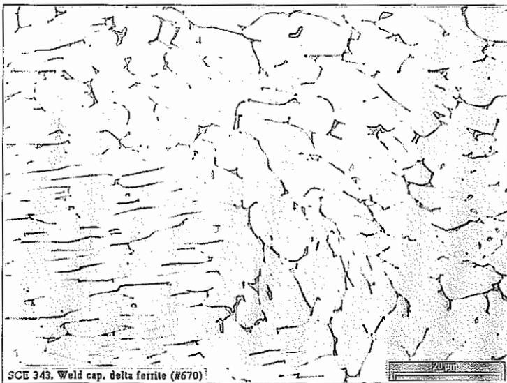
Figure 8  $\delta$ -Ferrite distribution in a 5 mm thick welded joint (unirradiated).
