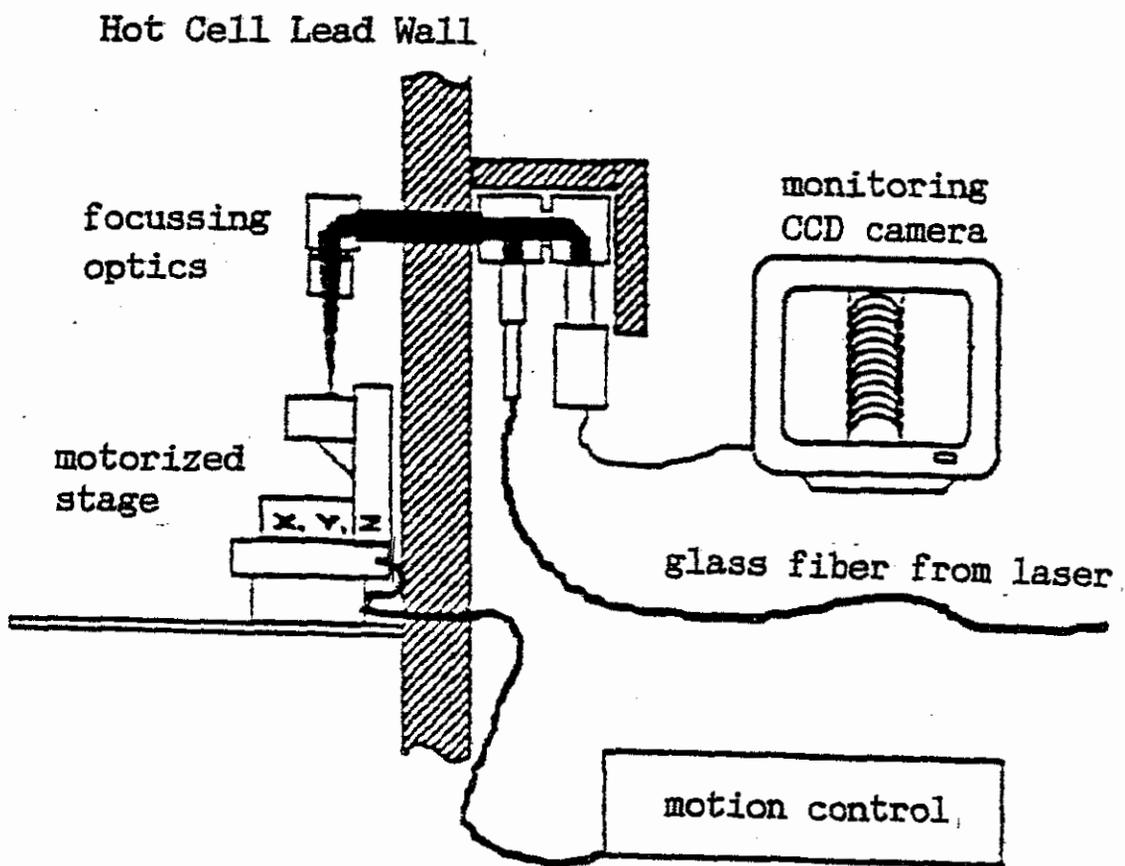
Figure 3 Schematic set-up of the laser welding equipment in the hot cell.
