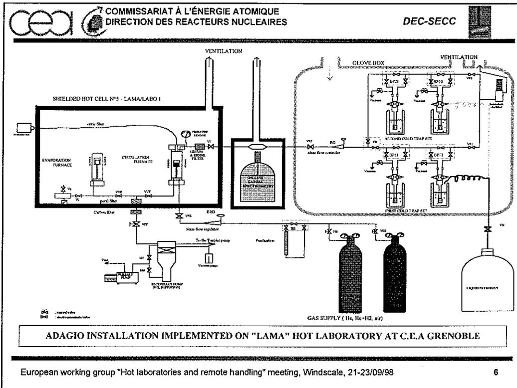
This schema describes all the equipments of the heat treatment device with on-line and cumulative gas release measurements. It could be divided in three main parts: the shielded hot cell, the gamma spectrometry monitoring and the glove box.
