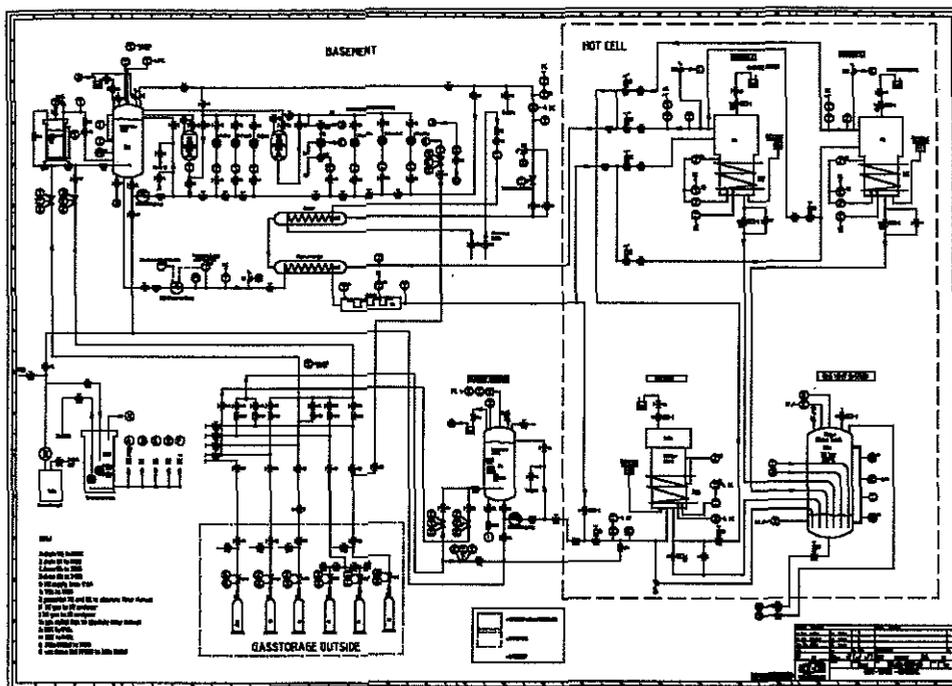
**Figure 3** Flow sheet of the test system: the low pressure part (top left corner), containing the water feed and storage tanks, the water chemistry monitoring and the the cleaning system; the high pressure section, containing the pump, heat exchangers and the autoclaves (left, inside the hot-cell); the conditioning and filling tank for the Hastelloy autoclave (lower center); the gas supply system (lower left) and the blow down tank, also inside the hot-cell (lower right).
