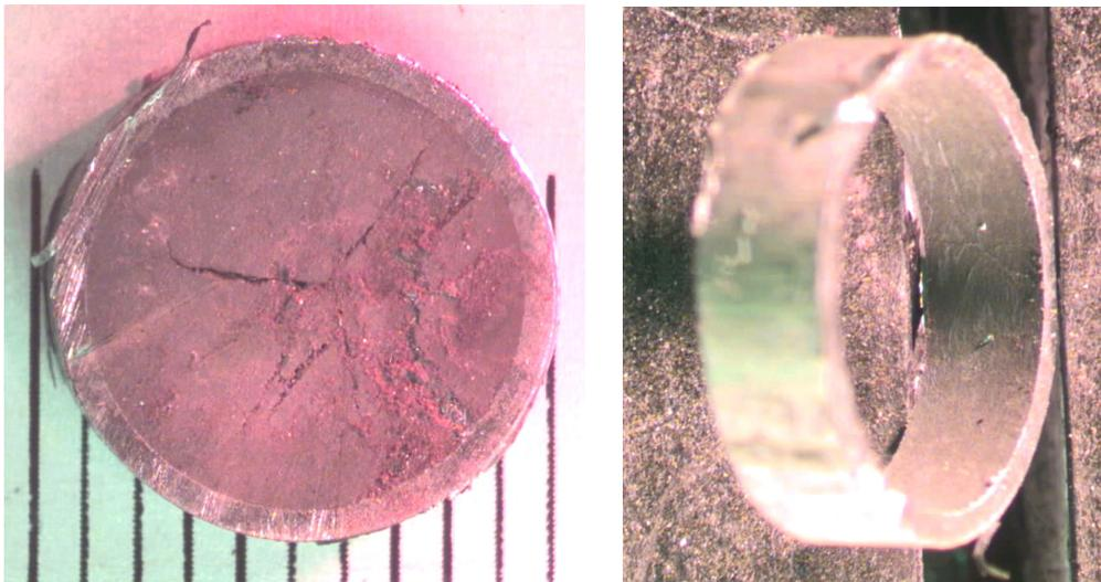
Figure 3 Fuel bonded to the cladding and the cladding after chemical fuel removal.
