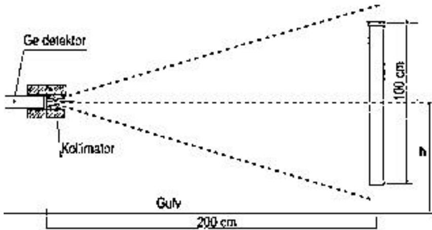
Fig. 6: Germanium detector focusing the basket
