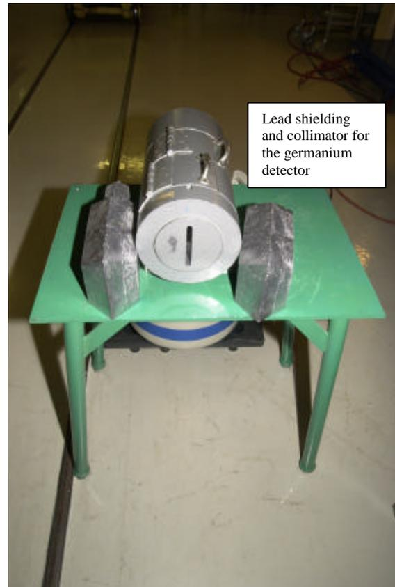
Fig. 8: Shielded collimator for the germanium detector
