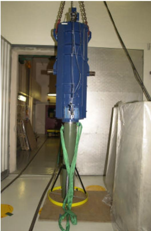
Fig. 9: The measuring arrangement with (blue) transport container and (green) basket container for gamma scan
