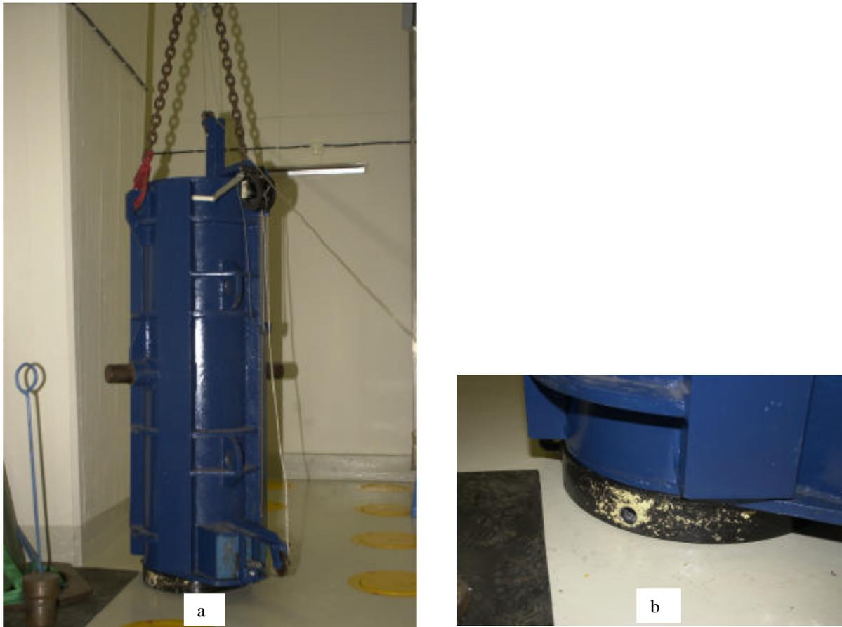
*Fig. 5: The transport container for lifting the standard baskets(a) and the inspection hole (b)*
