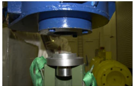
Fig. 10: Flange between the transport container and the basket container
