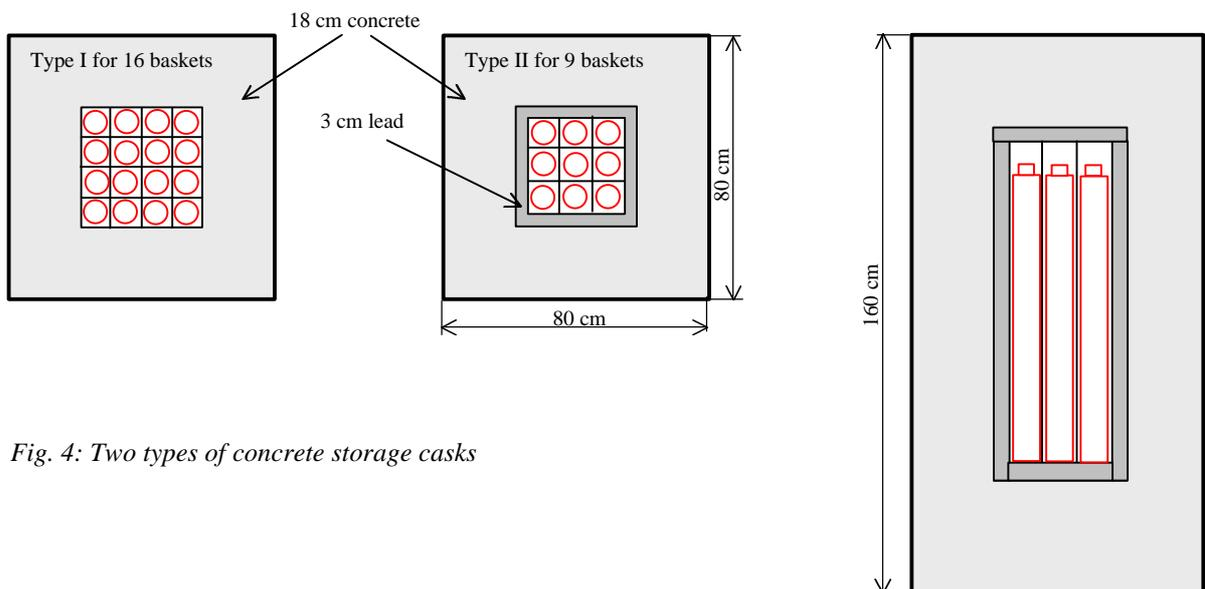
Fig. 4: Two types of concrete storage casks
