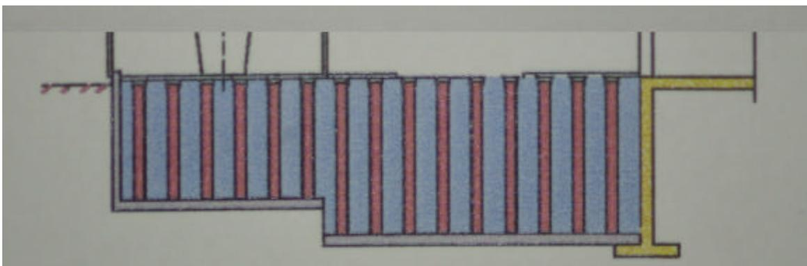
*Fig 3: Cross section of the pit store*
