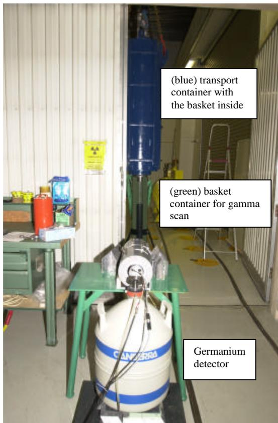
Fig. 7: Experimental set up for the measuring of  $^{137}\text{Cs}$  and  $^{60}\text{Co}$  with the germanium detector
