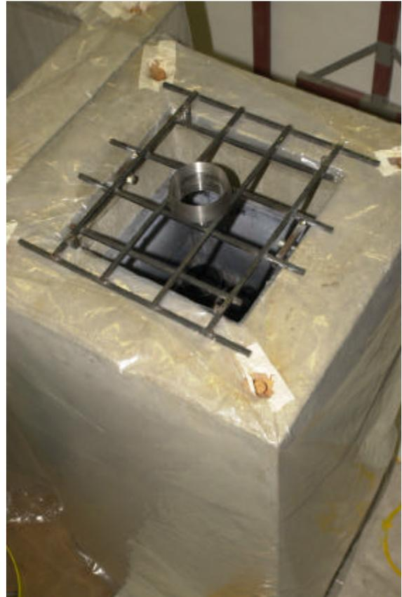
*Fig. 13: Concrete cask type II for 9 baskets. 18 cm concrete walls and 3 cm lead cladding*
