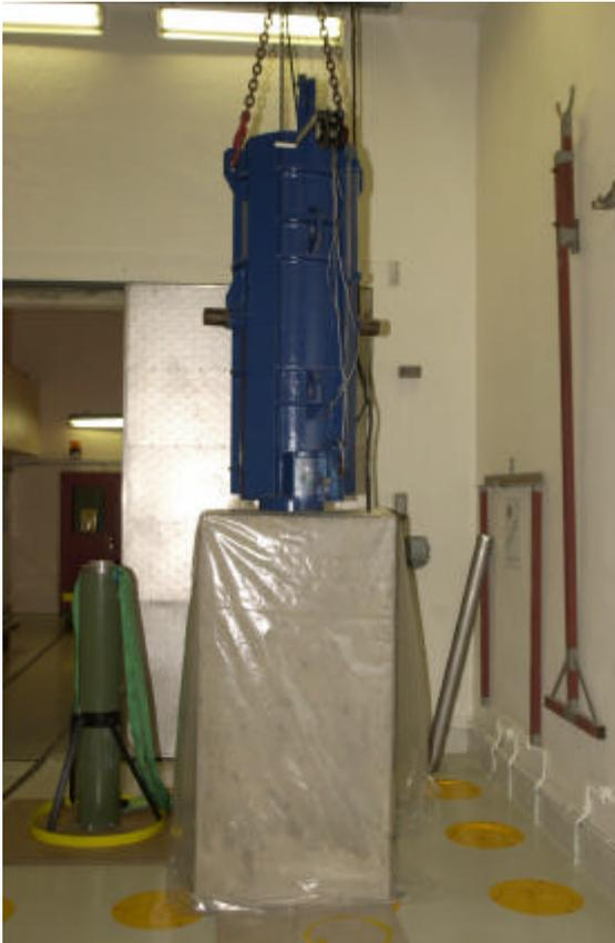
*Fig. 12: Transport container on top of the concrete cask.*
