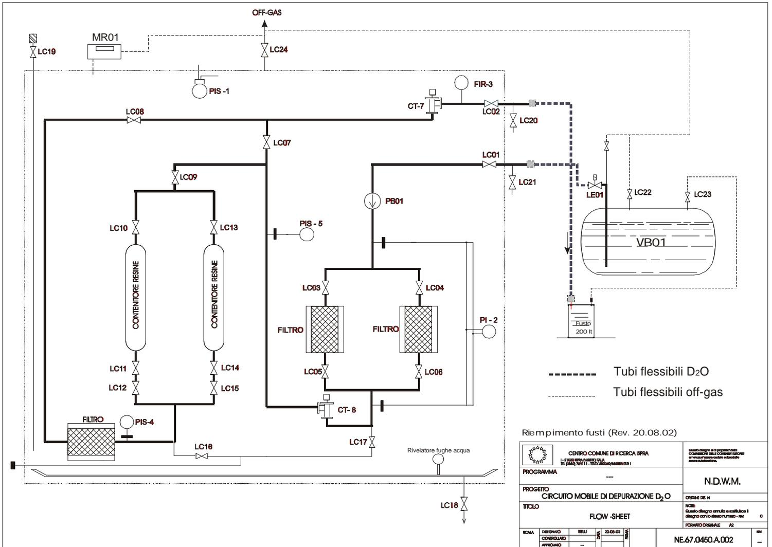
Fig. 2 – The mobile purification equipment filling the new drums with purified D<sub>2</sub>O
