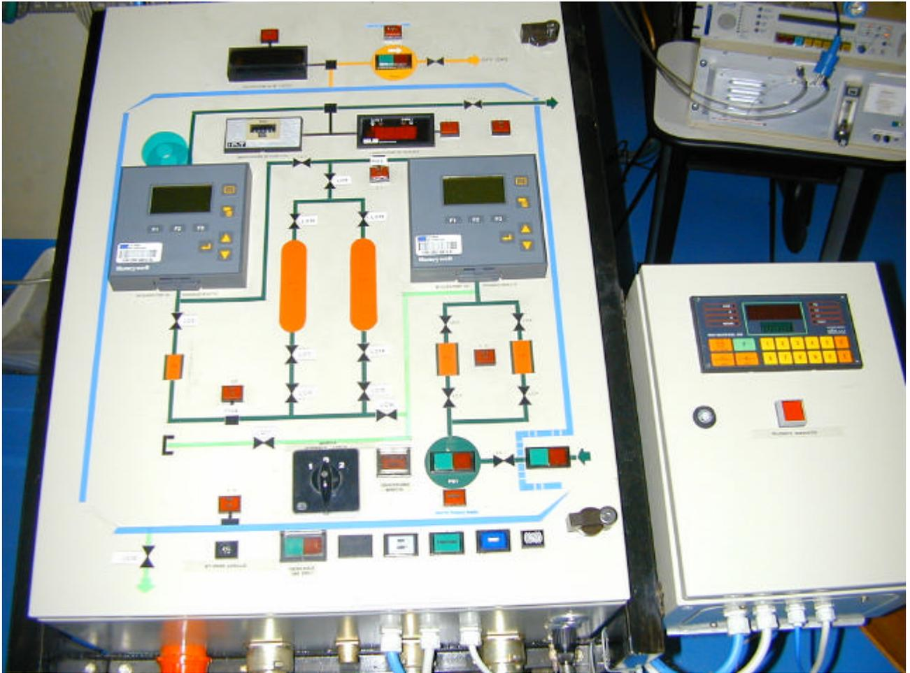
Fig. 5 – The control panel of the mobile purification equipment
