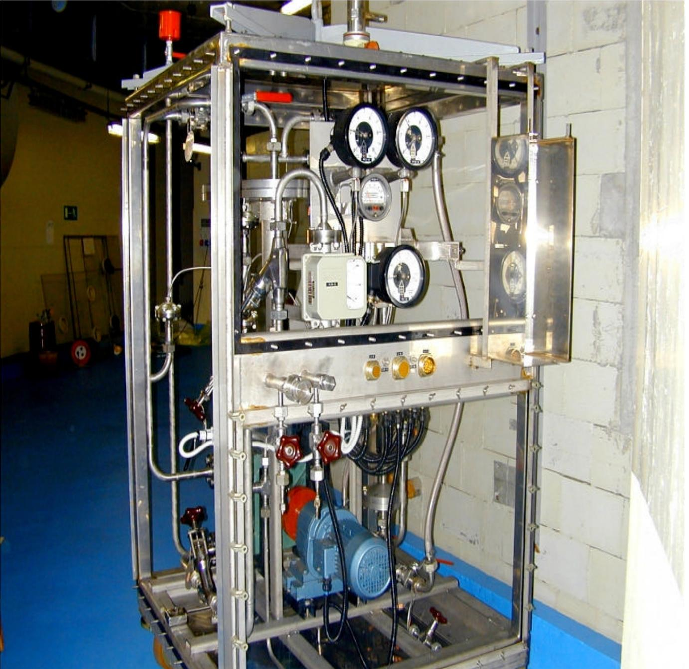
Fig. 3 – The mobile purification equipment
