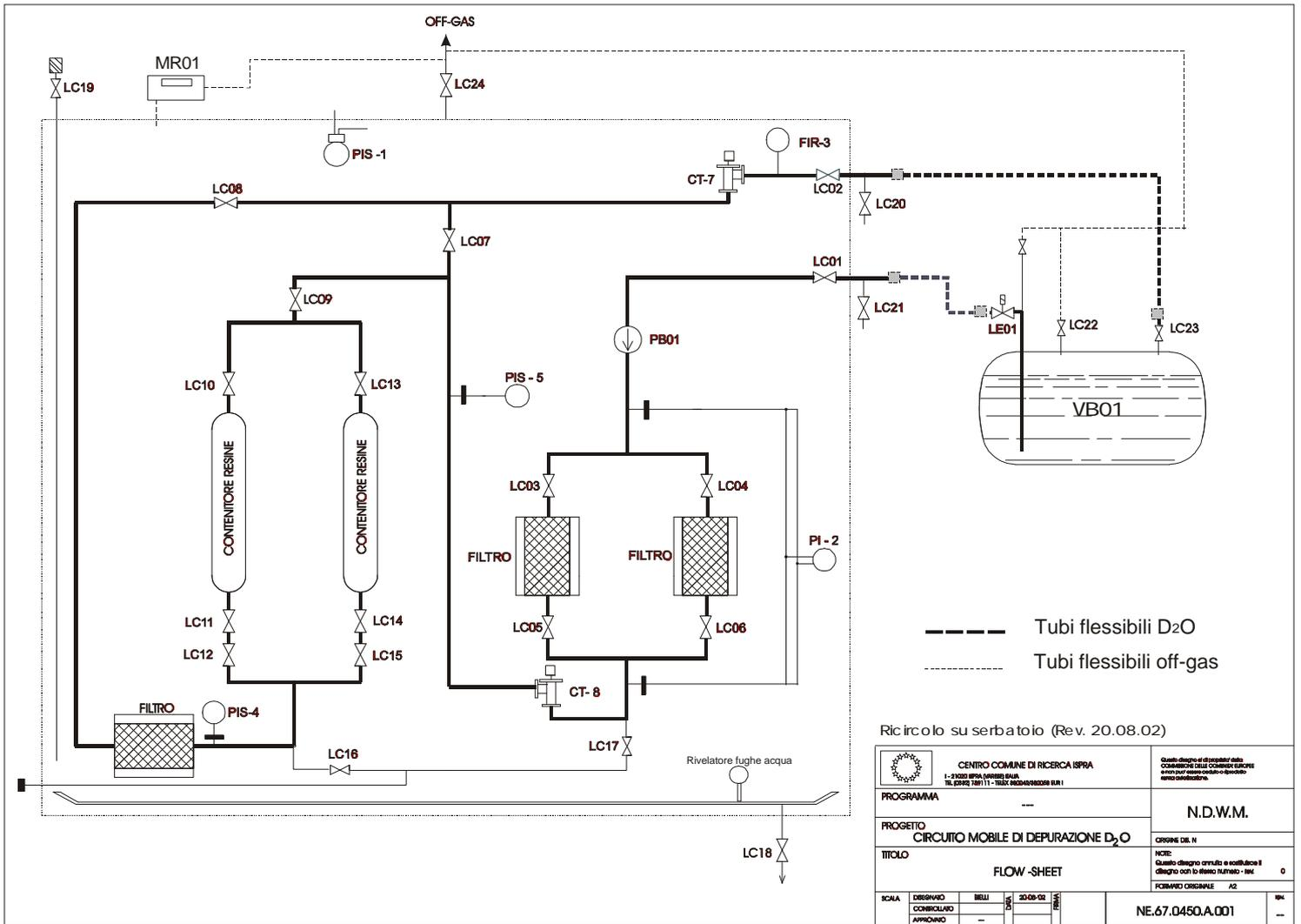
Fig. 1 – The mobile purification equipment recirculating the D<sub>2</sub>O into tank VB01
