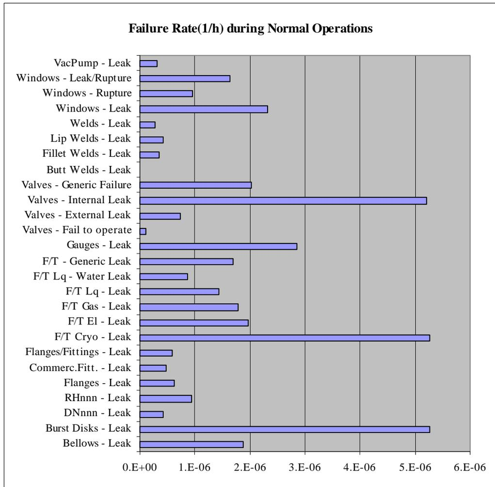
**Figure 5:** Failure rate (per hour of operation time) for each failure mode identified for the JET vacuum system.
