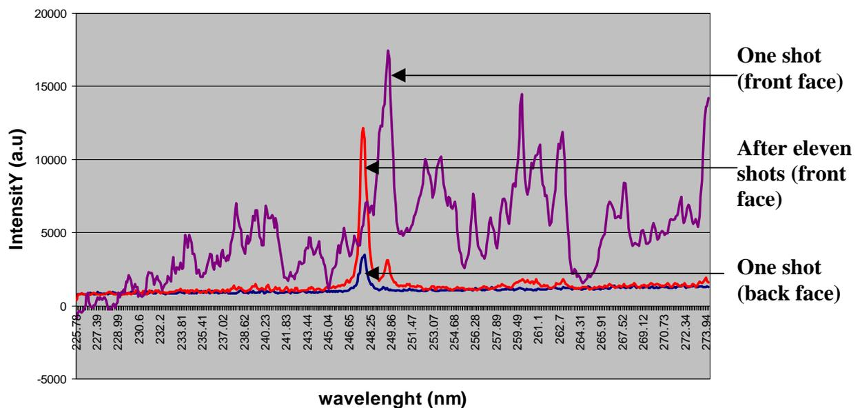
**Figure 3:** Optical Emission Spectroscopy of a carbon tile from Tore Supra before and after scanning with a laser to remove the co-deposited layer.
