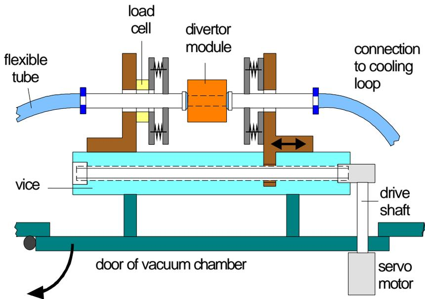
Fig. 2: Clamping system for water supply of actively cooled test modules
