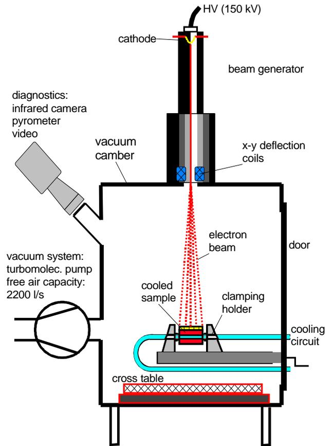
Fig. 1: Electron beam test facility JUDITH
