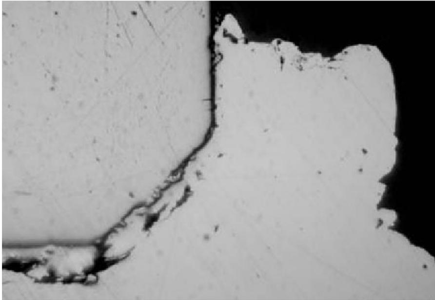
Fig. 6: Metallographic sectioning of an irradiated tungsten mock-up (1 dpa at 200°C) after testing under thermal fatigue conditions
