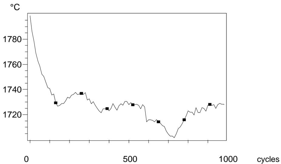
Fig. 4: Maximum temperature during thermal fatigue test of an irradiated CFC flat tile mock-up (irradiation condition: 0.2 dpa at 200°C)
