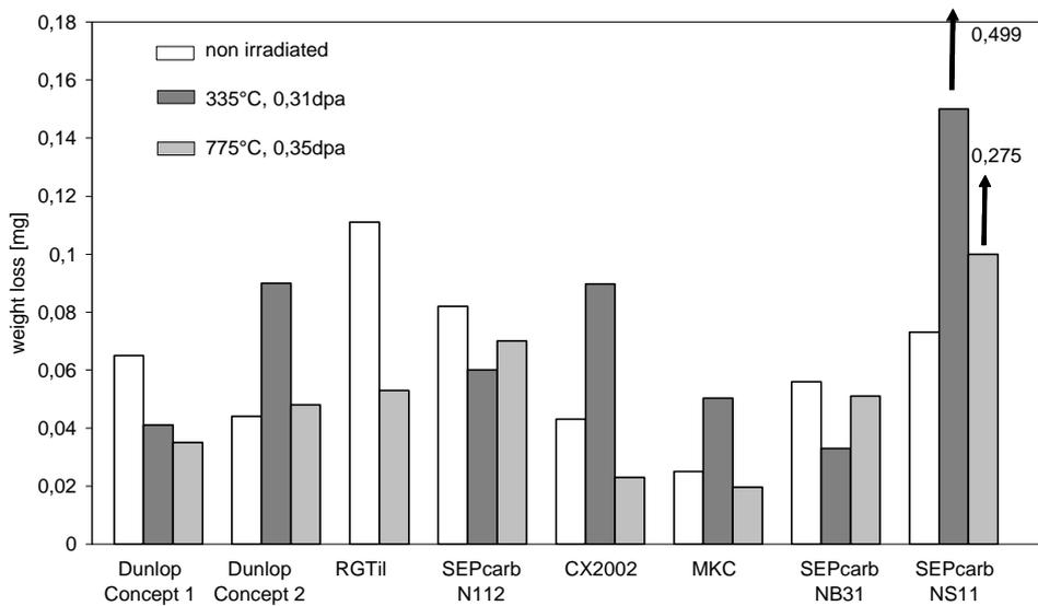
Fig. 7: Weight loss during thermal shock tests for different CFC materials
