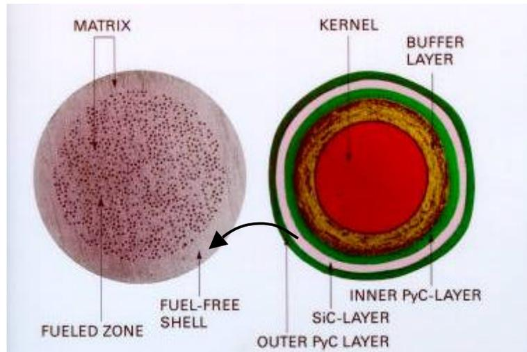
**Figure 1 :** *Cross-section of a pebble fuel element and HTR coated particle, source [1]*
