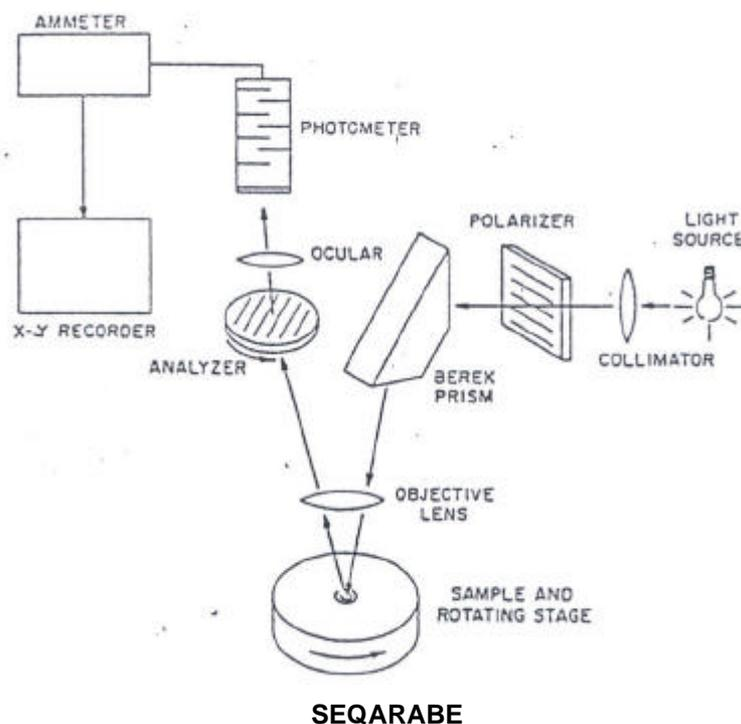
Figure 2 : Schematic showing principal elements of microphotometer [7]
