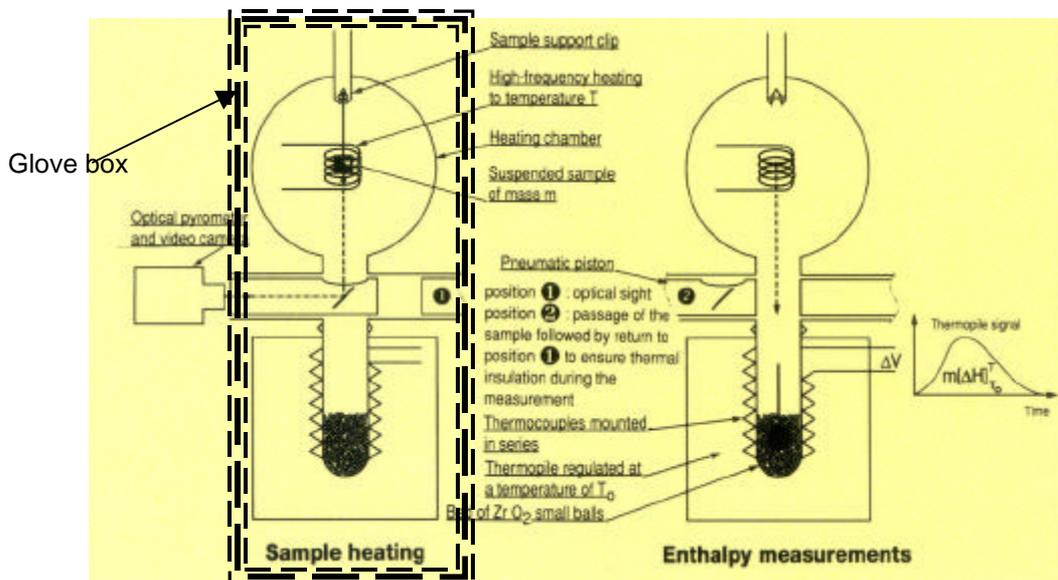
Figure 4 : Drop calorimetry configuration
