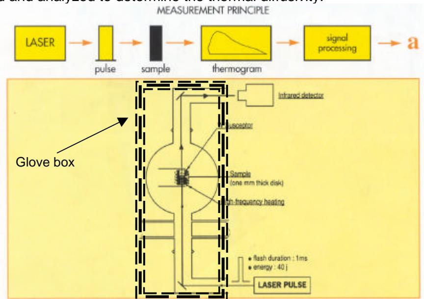
Figure 5 : Thermal diffusivity measurement configuration
