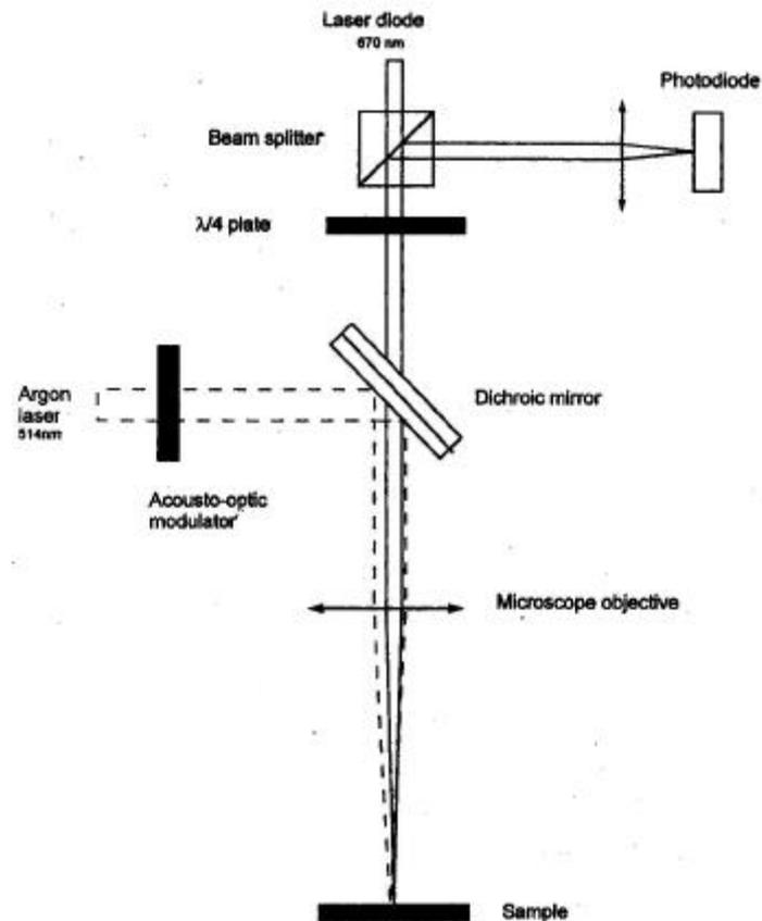
**Figure 6 :** *Sketch of the photoreflectance microscope*
