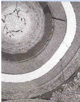
**Figure 7** : *irradiated HTR particle*
