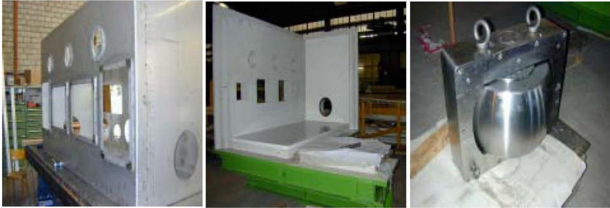
**Fig. 2** Picture of the inner alpha containment, of the steel shielding and of the large rotating lock during the construction of the box
