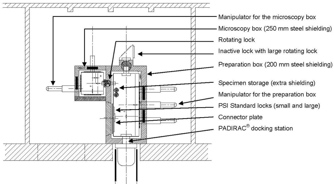
**Fig. 1** Sketch of the new PSI metallography box
