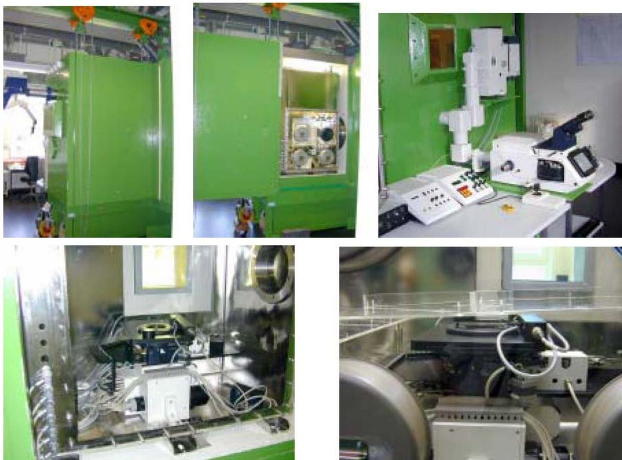
**Fig. 7** Up-left and centre: microscopy box with sliding door closed and open; Up-right: external part of the microscope; down-left: internal part of the microscope; down-right: upper part of the internal part of the microscope with its Plexiglas shield
