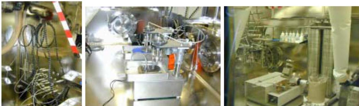
**Fig. 6** Left: connector plate and cable holders; middle: polishing machines; right: cutting machine
