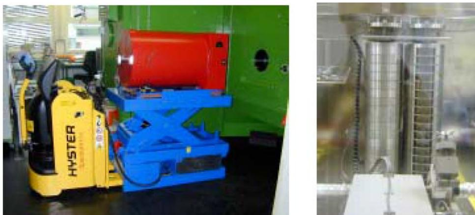
**Fig. 4** Left: shielded cask in front of the PSI lock for waste disposal; Right: internal shielded specimen storage
