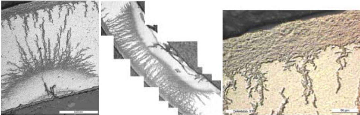
**Fig. 8** Observation of the hydride structure in an irradiated Zircaloy cladding cross section at different magnifications. The two left pictures have been realised by stitching two and 7 pictures together respectively
