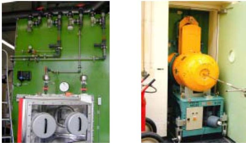
**Fig. 3** Left: under-pressure regulation and feeding systems for the boxes (upper part of the picture) and inactive lock for the transfer of consumables (bottom part of the picture); Right: PADIRAC cask docked on the box
