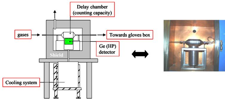
**Figure 3.** Online gamma spectrometry device, (a) schematic diagram and (b) photography
