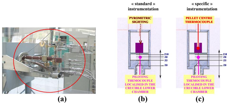
**Figure 2.** (a) Photography of the induction furnace, (b) scheme of the crucible with its standard instrumentation, (c) scheme of the crucible with its specific instrumentation
