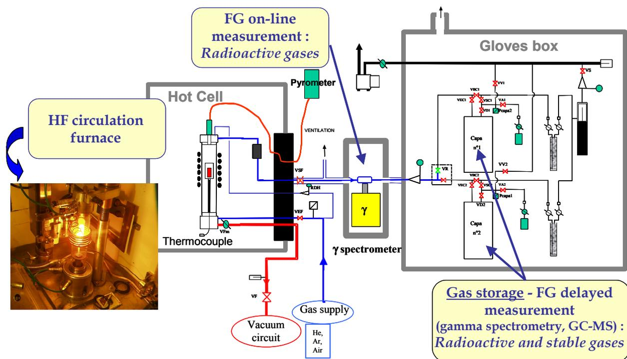
Figure 1. Simplified diagram of MERARG facility
