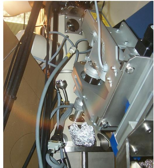
**Figure 6.** Schematic overview of the EPMA-MXRF instrument (left). The iMoxs module is mounted on the EDX port of the epma instrument (right)
