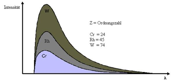
**Figure 3.** Intensity of bremsstrahlung increases with atomic number  $Z$  of the anode material.
