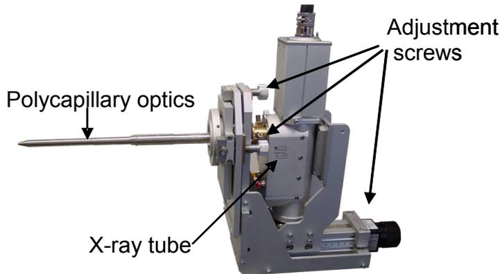
**Figure 7.** The iMOXS module consists of a tungsten X-ray tube and polycapillary optics to transfer and focus the X-rays on the sample
