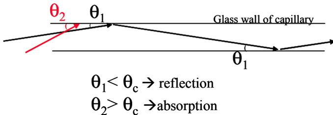
**Figure 4.** Total external reflection of X-rays.
