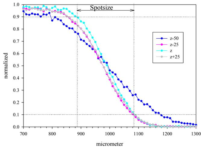
**Figure 8.** Measurement of the spot width generated by 6.4 keV photons emitted by the sample
