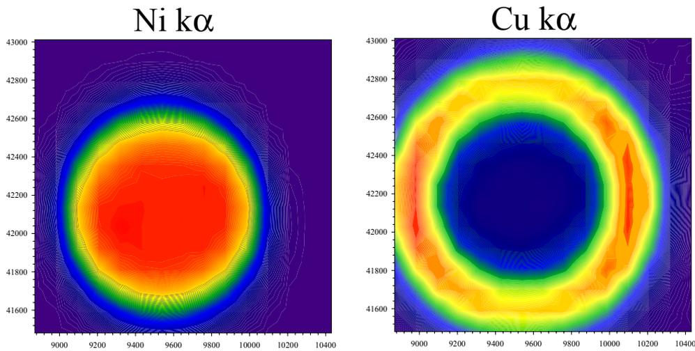
**Figure 9.** Mapping of a Cu-Ni target using a 200 mm spot. The X and Y axis are in  $\mu\text{m}$  units
