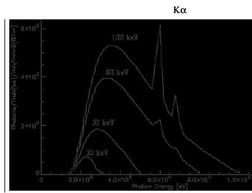
**Figure 2.** Influence of applied voltage on X-ray tube spectrum
