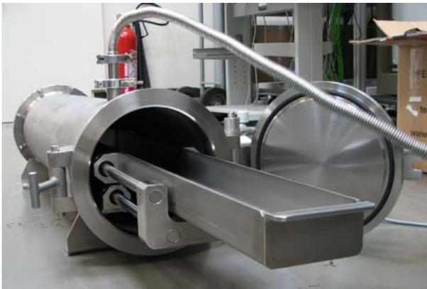
**figure 4:**      Vacuum chamber of leak-testing set-up.
