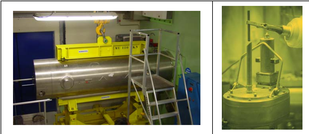
Figure 1. TN106 cask connected on the shielded process line
