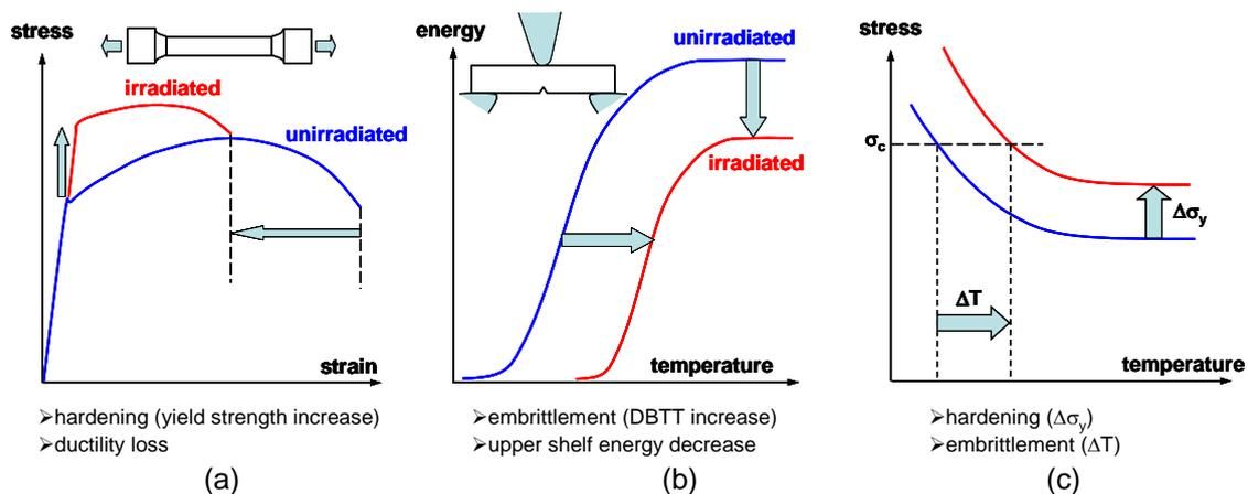
**Figure 2.** Illustration of irradiation-induced hardening and embrittlement.
