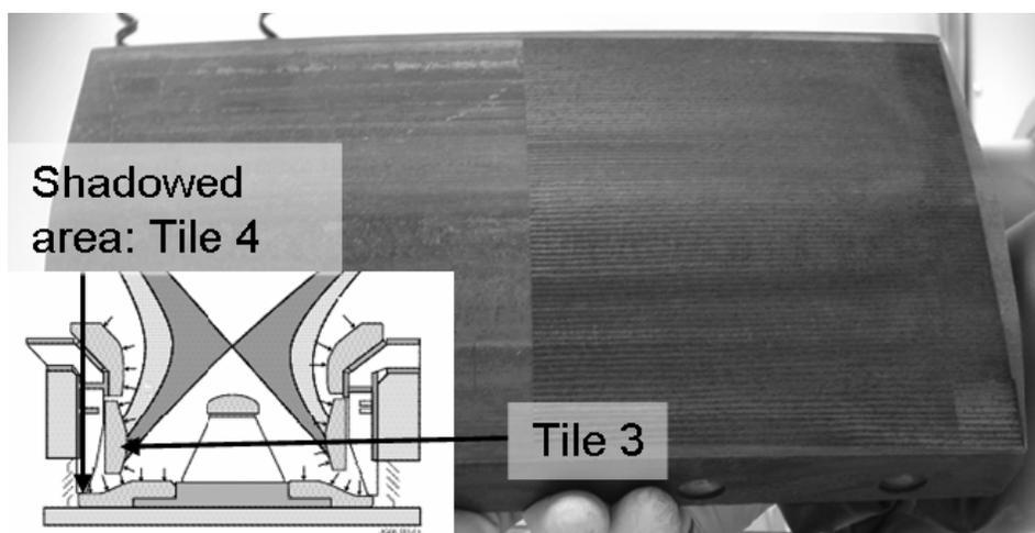
**Fig.1.** Shows tile G3B14IN after half of the surface has been laser cleaned. Fibre planes are visible on the right hand side of the tile photograph. The insert shows the positions of tile 3 and tile 4 in the JET MkIIIGB divertor.
