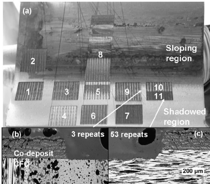
**Fig.2a.** Photograph showing areas cleaned on tile G4A5BW using different scanning regimes. Figs. 2b and 2c show cross-sectional micrographs at the interfaces indicated by the arrows.
