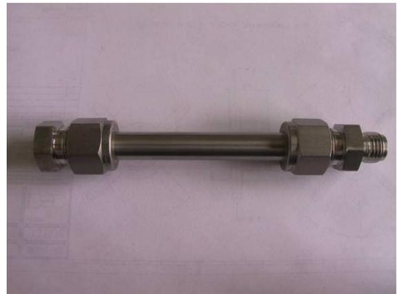
**Figure 2:** I-SCC specimen (90mm in length), left picture: de-fuelled cladding tube and Swagelok union and end plug, right picture: de-fuelled cladding tube with connected Swagelok union and end plug
