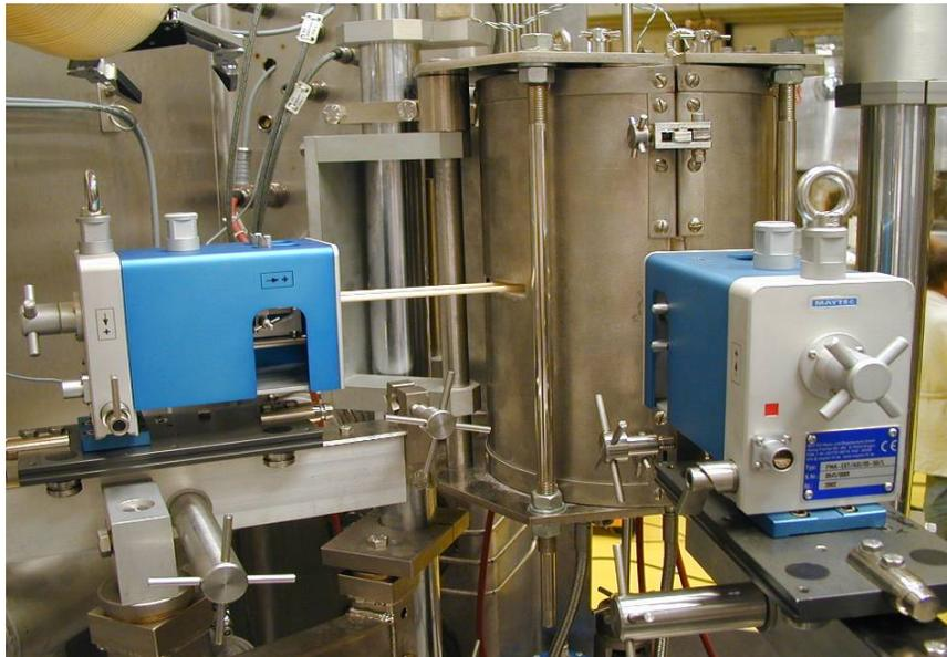
**Figure 6 :** View of one of the two machines from inside of the cell, notice the diametrical and the axial extensometers in the blue aluminum boxes and the zircon rods passing through a slot machined in the furnace
