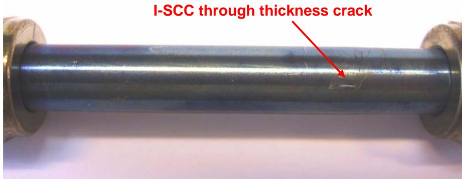
**Figure 3 :** Picture of a 90mm I-SCC cladding specimen in un-irradiated recrystallized Zircaloy-4 showing through thickness cracking after testing at 350°C and  $10^{-5} \text{ s}^{-1}$  constant strain rate
