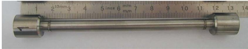
Figure 7 : Cladding specimen with laser beam welded end-plugs for axial creep testing
