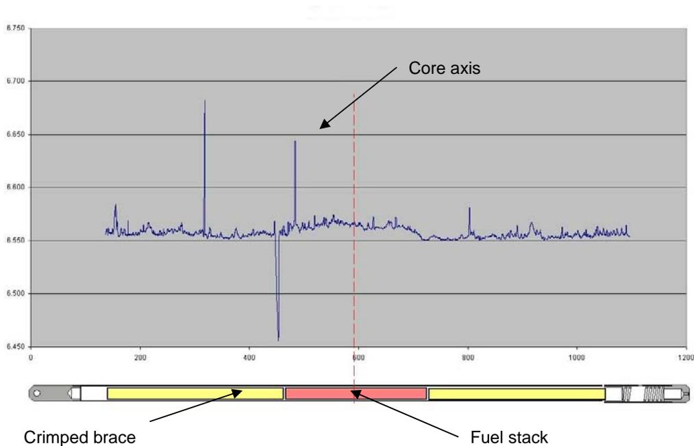
**Fig. 6:** Pin diameter measurement
