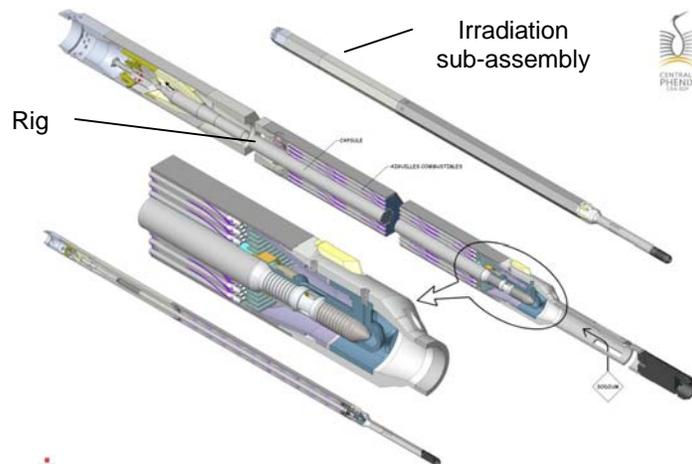
**Fig.5:** Rig inside a carrier
