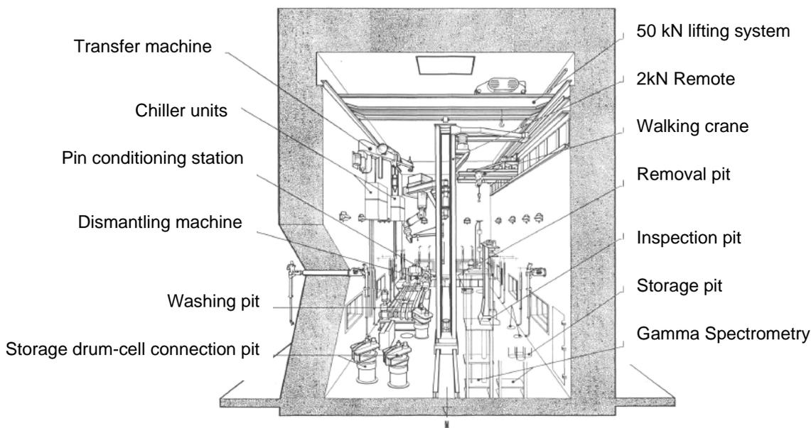
**Fig.1: The Irradiated Elements Cell**
