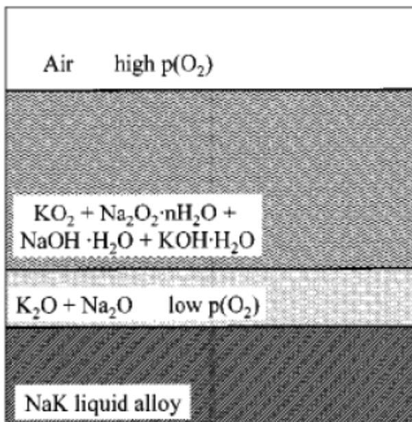
With such a model, it has been possible to identify the starting event of accidental explosions occurred in the past during handling operations on NaK at room temperature: the accidental contact of the external super oxides layer with the underneath liquid metal alloy.
