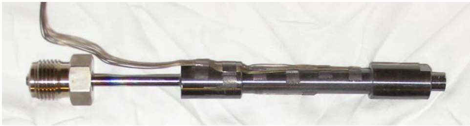
Fig. 9 Sample for adjustment of temperature of the furnace coils.
