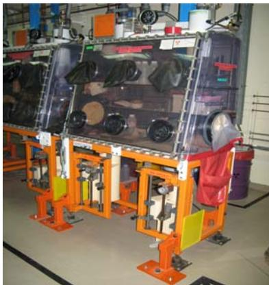
Fig 1 : Anchoring the glove base to the floor and interlocking its framework with the containment box
